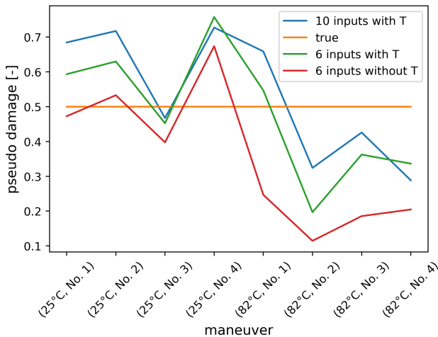
Figure 6: Pseudo damage of the TS predicted by the ML models compared to the original TS.
