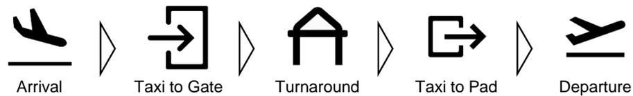
**Figure 2.8:** Process steps at a vertiport for an eVTOL [88]
