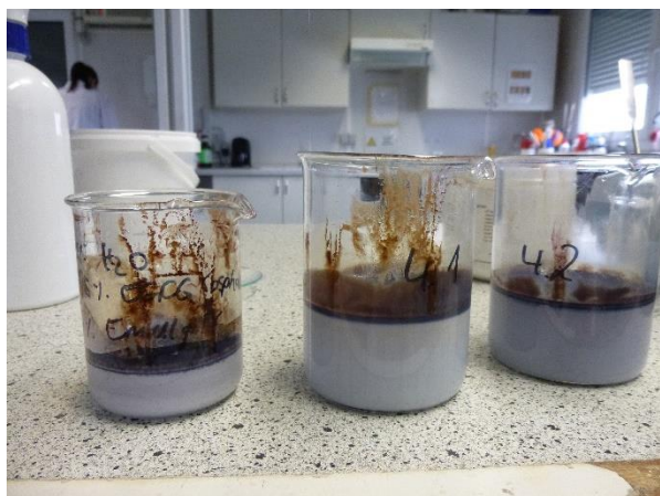
Figure 1: Unstable solutions; change in formulation color (white to brown) after 1h at room temperature
