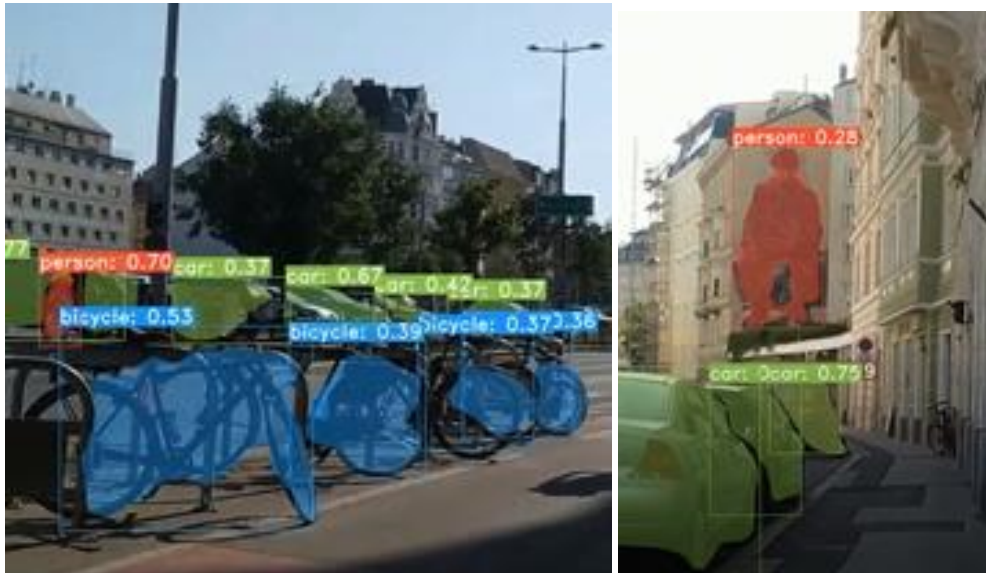
(a) Deformed instances (b) Misclassification Figure 17. Limitations of YOLACT such as (a) deformed instances and (b) misclassification.
