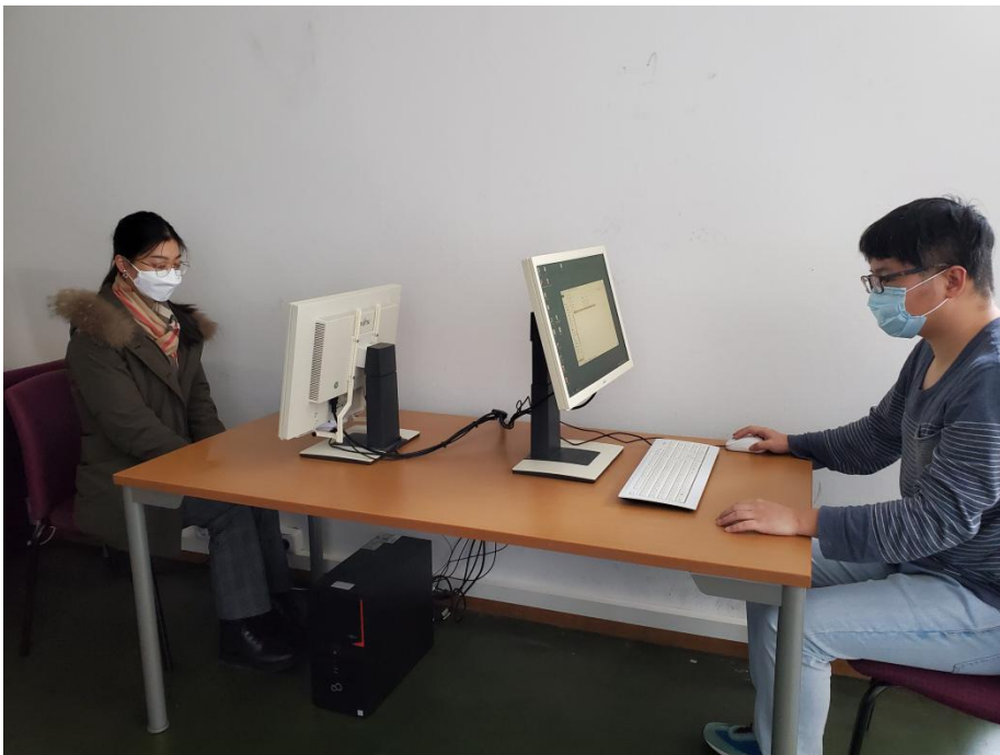
Figure 5. A Picture Showing the Experiment Environment. (A participant (left) was doing the eye-tracking experiment with the Gaze Point GP3 eye tracker, while a controller (right) was observing the eye and mouse movements of the participant on another screen.)
