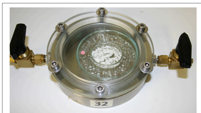
FIGURE 1 | Experimental setup for the oxygen absorption measurements.
