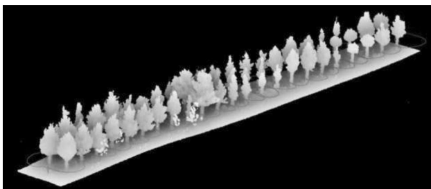
Fig. 2 Exemplary picture of trees of two rows after processing a mobile scan in GeoSlam Hub. The red line indicates the trajectory of the device during scanning with the loop being closed for each scan at the front left (start and end at beginning of row). Two tree rows were always scanned at a time by a zig-zagging walking path trajectory surrounding each tree in the two rows
