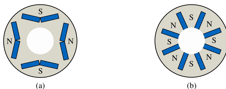
Figure 2.3: General structure of IPMSMs. (a) Interior permanent magnet synchronous machine. (b) Interior permanent magnet synchronous machine (with circumferential orientation).
