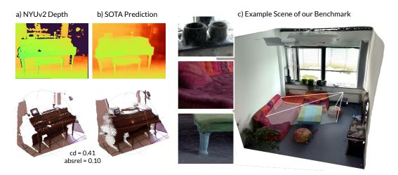
**Fig. 3.14.** b) State-of-the-art depth prediction with low absolute relative error often do not exhibit correct 3D structures when back-projected in 3D space. We suggest to use 3D metrics to measure the quality of the prediction and propose d) a new depth prediction benchmark with full 3D geometry and high quality depth compared to raw sensor measurements (a) [207].
