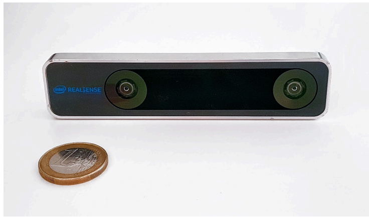
Figure 1.6.: The Intel® RealSense™ T265 tracking camera. The device features two fish eye cameras, an accelerometer, and a gyroscope and runs a VI-SLAM algorithm in real time on a dedicated chipset to produce a pose estimate at 200 Hz.
