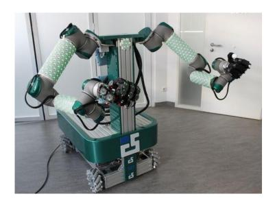
Figure 2 Experimental platform TOMM, semi-humanoid robot with two 6-DOF arms covered with artificial skin.
