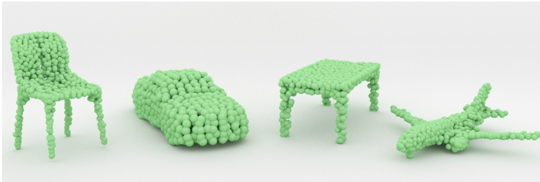
Figure 2.1: Point Cloud Representation. Point cloud can be used to represent 3D geometry of different shapes [15], such as table, chair etc.
