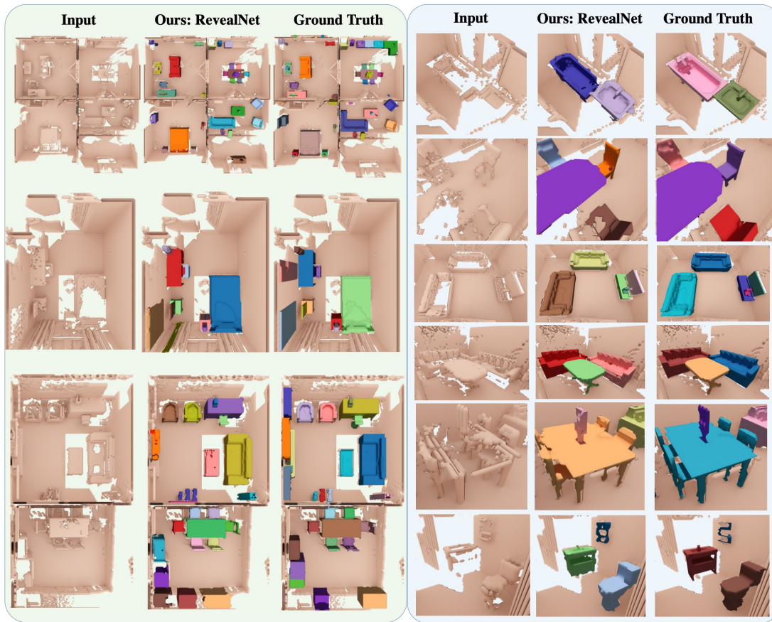
Figure 4.4: Qualitative results on SUNCG dataset [17] (left: full scans, right: close-ups). We sample RGB-D images to reconstruct incomplete 3D scans from random camera trajectories inside SUNCG scenes. Note that different colors denote distinct object instances in the visualization.
