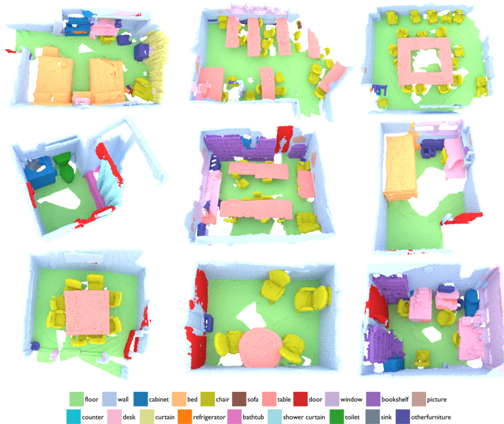
Figure 5.10: Semantic Segmentation Results (ScanNet-LA). With our pre-trained model as initialization for fine-tuning, together with an active labeling process, our approach generates high-quality semantic segmentation predictions. Here our model is fine-tuned with 20 labeled points per scene.
