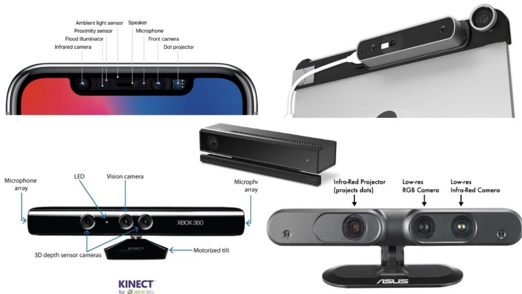
Figure 1.1: Depth Sensors on the Market. Commodity 3D Sensors are now readily available on the market from a variety of companies. Portable sensors are easily mounted on mobile devices and carried around for collecting data.
