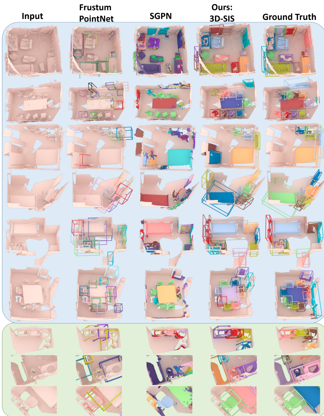
Figure 3.3: Qualitative comparison of 3D object detection and instance segmentation on ScanNetV2 [4]. Full scans above; close-ups below. Our joint color-geometry feature learning combined with our fully-convolutional approach to inference on full test scans at once enables more accurate and semantically coherent predictions. Note that different colors represent different instances, and the same instances in the ground truth and predictions are not necessarily the same color.
