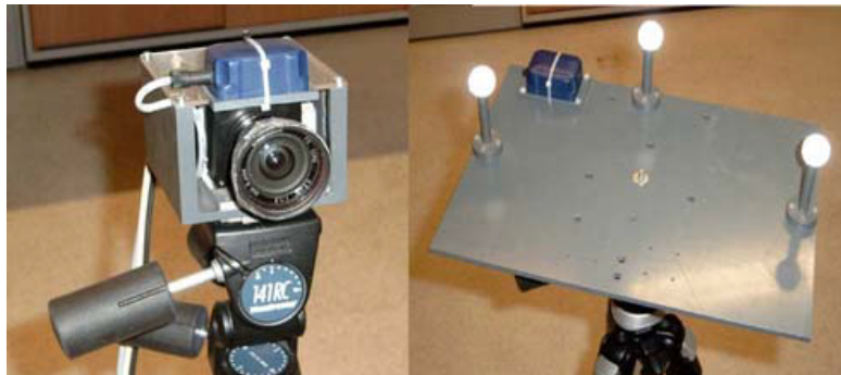
Figure 6.3.: Hybrid setups: inside-out tracker (left) and outside-in tracker target board (right). Source: [156]
