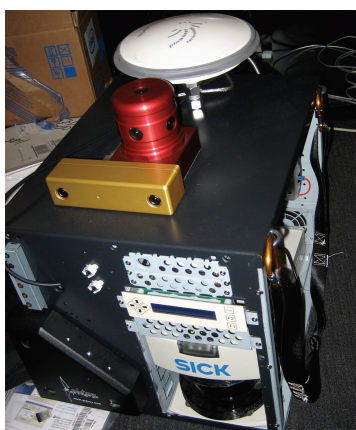
Figure 6.7.: Experimental setup: monocular camera and IMU. Source: [135]
