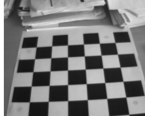
Figure 4.14.: Visual pattern used for joint Camera-IMU calibration. Source: [295]
