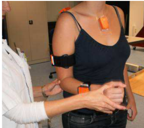
Figure 10.6.: Components of Xsens body sensor network placed on the body. Source: [218]
