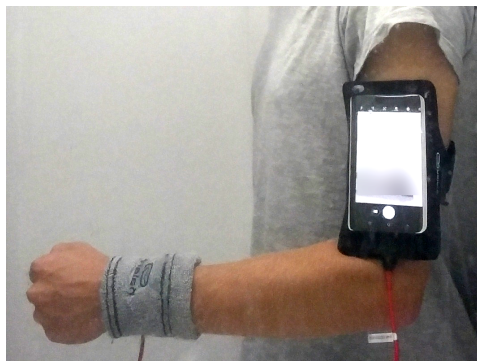
Figure 10.13.: The sensor network consisting of a smartphone and an Arduino Sensor. Source: [205]
