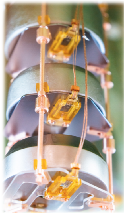
Figure 11.5: Photograph of a detector string in the Post- GERDA Test. Image courtesy of M. Willers.
