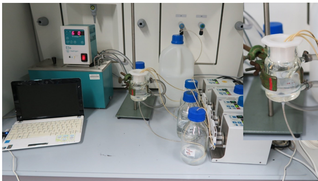
Figure S3: Experimental setup for the LPE process. For the thin film deposition, a double-walled reaction vessel, which was heated with a silicon-oil thermostat was used. The solutions were pumped in and out by peristaltic pumps computer controlled by LABview. The substrate was placed in the double walled reaction vessel.
