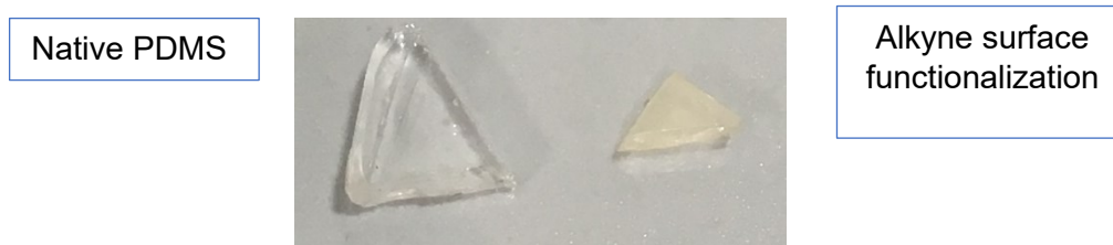
Figure S8: PDMS samples after performing the Baeyer test for free alkyne groups. Left: Native PDMS illustrating no colour change. Right: Surface functionalized with (3-chloropropyl)trimethoxysilane, subsequently converted to an alkyne group with sodium acetylide and a slightly brown colouring visible.
