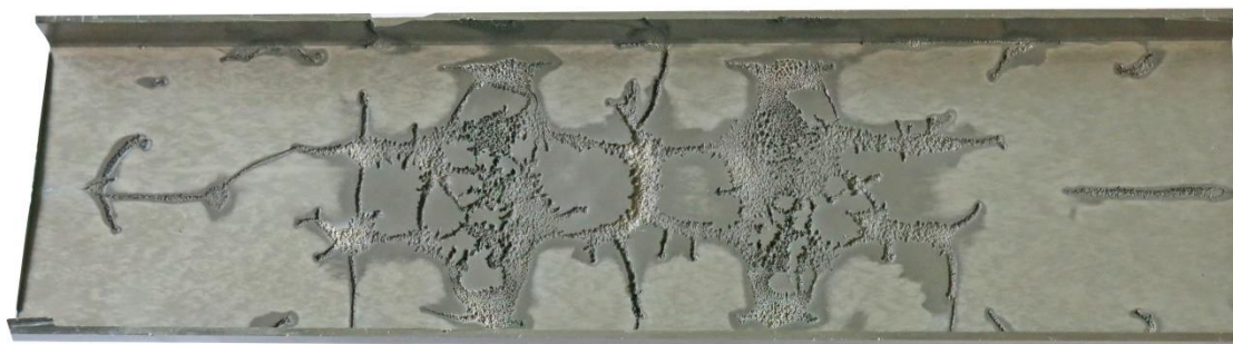
Figure 33: Example of cavitation erosion in a rectangular ultrasonic reactor with a gap size of 25 mm.
