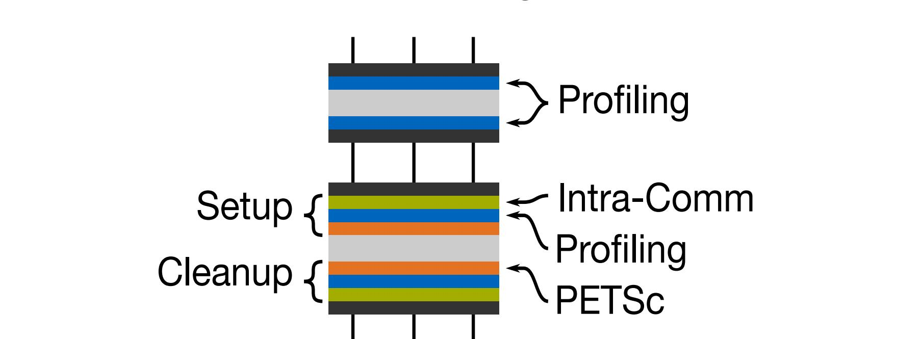
Requirements enable setup before and cleanup after tests. Top requires profiling, bottom requires PETSc & Intra-communication.
