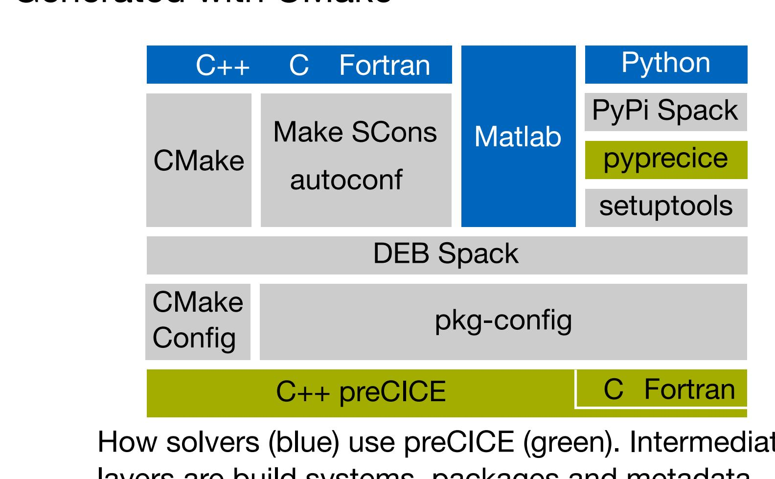
How solvers (blue) use preCICE (green). Intermediate layers are build systems, packages and metadata.
