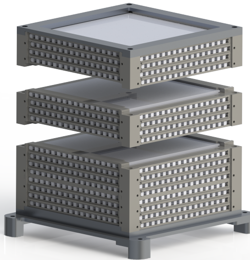
Figure 2.2: ADU of the RadMap Telescope: Exploded view of the fiber stack shows the alignment and sectioning.
