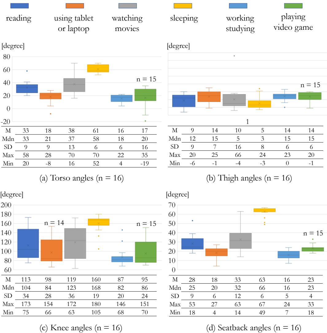
Figure 4-3 Joint angles and seatback adjustments of NDPs in different NDRTs, modified from (Yang et al., 2019)
