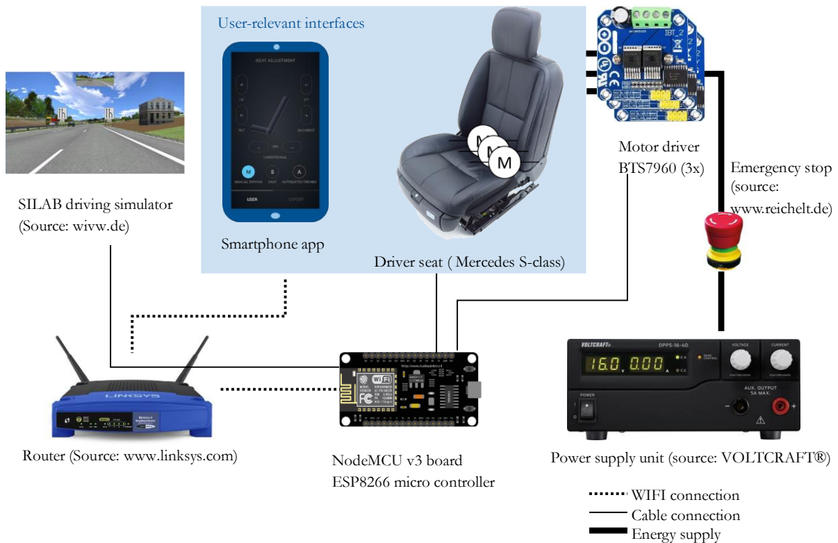
Figure 7-2 The system structure of the active seat assist prototype, modified from Wolf (2018)
