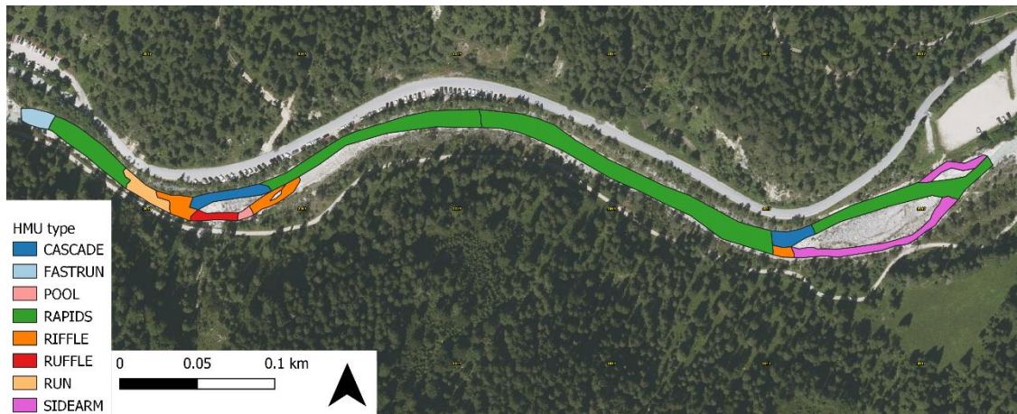
Figure 35 HMU types identified during a discharge of 2.39 m 3 /s on 3 rd September 2019 at River Leutasch
