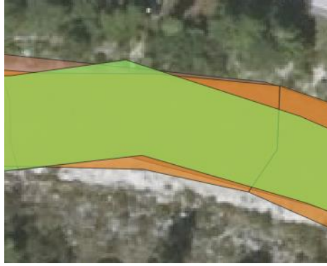
Figure 28 HMU-polygons based on the GPS coordinates (green 19.12.19, 0.6 m 3 /s; orange 27.8.19, 1.8 m 3 /s; red 3.9.19 2.3 m 3 /s)
