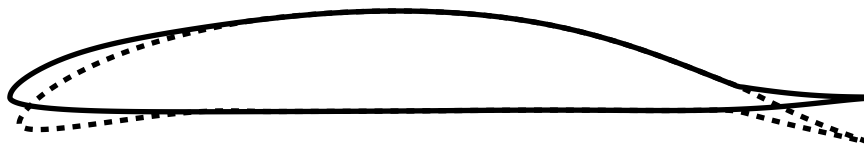
Figure 1.1: Laminar airfoil with droop nose and trailing edge flap (Weinzierl et al. 2015).
