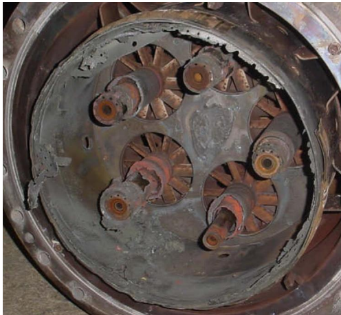
Figure 1.1: Damages of a combustor face plate due to thermoacoustic instability. 1
