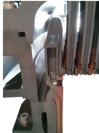
Figure 1.2: L-shaped quarter-wave resonator in a Vulcain 2 engine. 2
