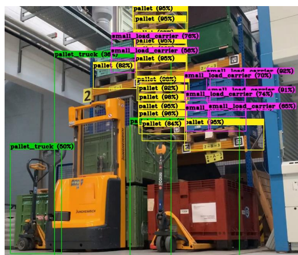
Figure 6: Optical identification of logistics specific objects in industrial environments [56]
