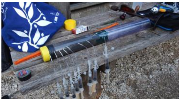
Figure 2.4 Pore water sampling (Lake Oberer Soiernsee)
