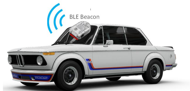
Figure 4.11: Location of the beacon in the vehicle (BMW Niederlassung, 2020)
