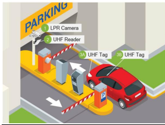
Figure 2.19: The main components of LPR system (ZKTECO, 2018)
