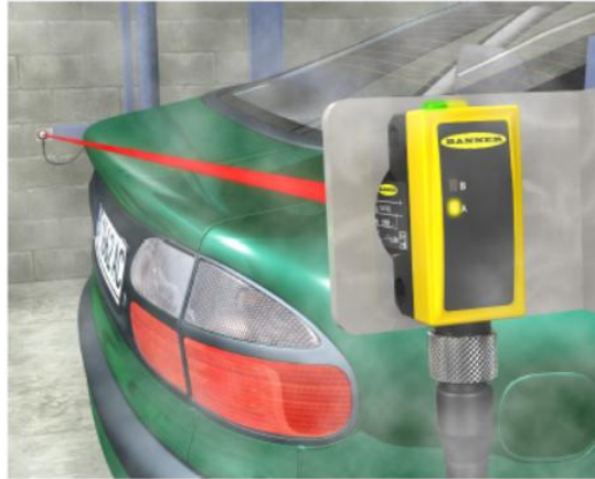
Figure 2.8: Vehicle detection using infrared optical at exit from a car wash (Banner Engineering Corp., 2017)
