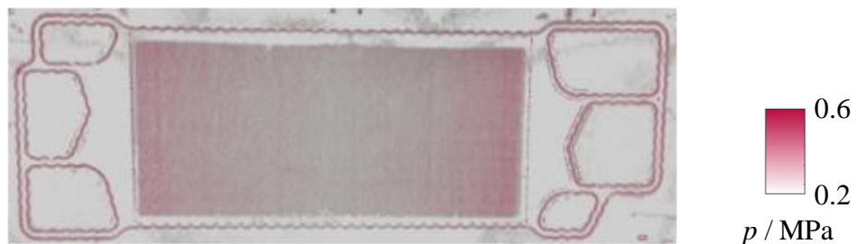
Figure 3.4. A) Functional areas of the bipolar plate for automotive fuel cells. B) Contact pressure distribution measured between the current scan device and the bipolar plate of the cathode according to Figure 3.3 .
