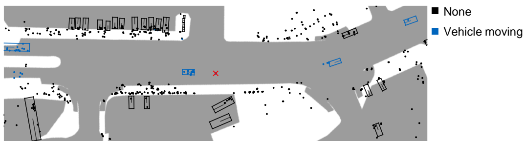
Figure 5.7: Example prediction of the KPLSTM model to differentiate moving vehicles from the surroundings. The point colors represent the actual model prediction, whereas the bounding boxes represent the ground truth data. This result is achieved on dynamic vehicle dataset.
