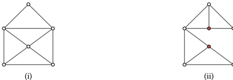
**Figure 6.2:** Depiction of a conforming (i) and non-conforming (ii) triangular mesh: red vertices indicate non-conformity.
