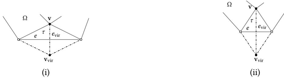
**Figure 8.13:** The concept of virtual edges: the virtual edge  $e_{\text{vir}}$  helps to push  $\mathbf{v}$  away from  $\partial\Omega$  (i). The triangle  $\tau$  is perfectly shaped for  $\|e_{\text{vir}}\| = \sqrt{3}\|e\|$  (ii).
