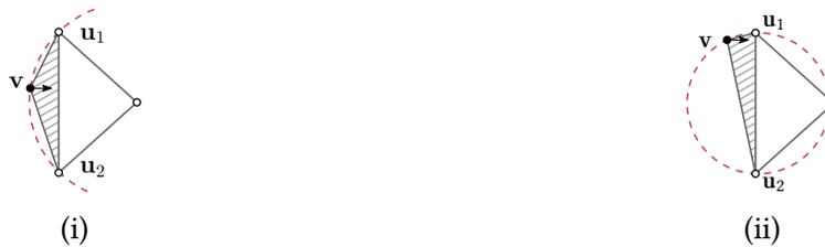
**Figure 8.5:** The two cases of an edge crossing vertex: the vertex does not move towards  $\mathbf{u}_1$  or  $\mathbf{u}_2$  (i). In that case, a large circumradius eventually leads to an edge flip. In the second case, the vertex moves towards  $\mathbf{u}_1$  (ii). This leads to a strong repulsive force between  $\mathbf{u}_1$  and  $\mathbf{v}$ , preventing  $\mathbf{v}$  from collapsing into  $\mathbf{u}_1$ .
