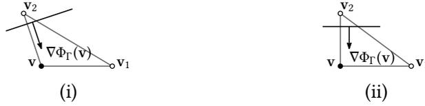
**Figure 9.3:** Causality violation caused by obtuse angles: for obtuse angles (i) it is possible that the wavefront (approximation), indicated by the black line, reaches either  $v_1$  or  $v_2$  but not both before it reaches  $v$ . For an acute triangulation this is impossible (ii).
