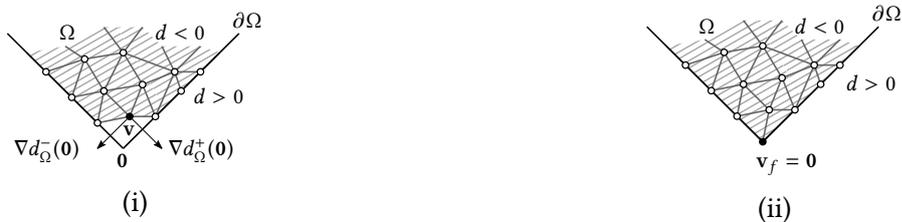
**Figure 8.8:** A problematic boundary which is difficult to adhere to since  $\nabla d_{\Omega}(\mathbf{0})$  is not uniquely defined (i). A fix point inserted at  $\mathbf{0}$  resolves the issue (ii).
