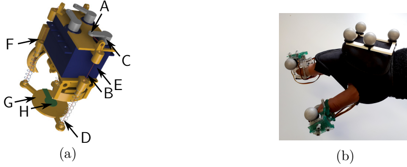
Figure 4.6: The actuated fingertip device. (a) A rigid body, A, houses three servomotors, E, connected via three tensors, B, to the vertices of the slanting platform, G. The platform is located under the finger pulp of the user whose distal phalanx holds the fingertip in its position with a clamp, F. A force sensor, H, is located on the platform, under the finger pulp center. The initial position of the platform is held by three springs, D. (b) The hand setup with the fingertip devices and passive markers.
