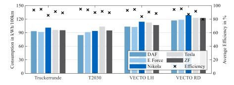
**Figure 5.** Varying driving cycles with different characteristics have an influence on energy consumption and average electric machine efficiency. While Truckerrunde and T2030 do not include stops, both VECTO cycles include multiple stops with varying times (LH: 67 s and RD: 746 s). The spreadsheet containing the results is provided as Supplementary Material.
