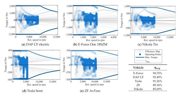
**Figure 4.** Simulation results of operating points, maximum, and average efficiency for regarded electric truck concepts (**a**–**e**) during the *Truckerrunde* driving cycle. The hyperbolic shapes are caused by the technical, maximum current of 500 A.
