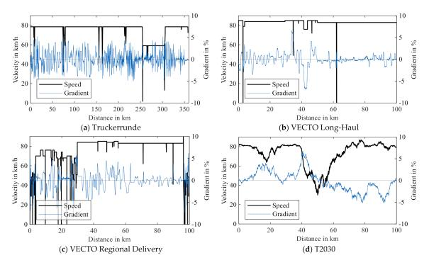
**Figure 2.** Speed profile and road gradient of different driving cycles (**a**–**d**). *Truckerrunde* is based on a real road-profile, while the other driving cycles are synthetic driving cycles based on collected and processed driving data.
