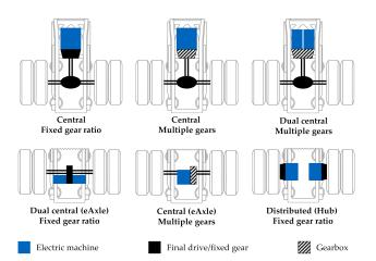
Figure 1. Topologies for electric drive axles for heavy-duty trucks.
