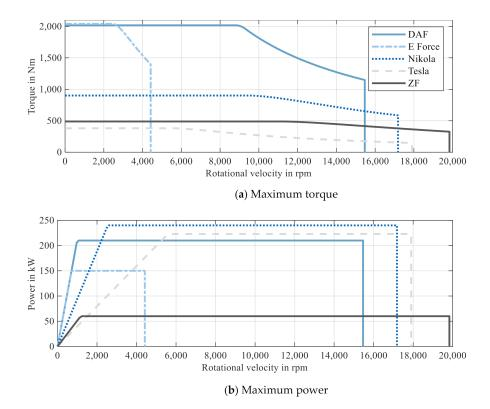
**Figure 3.** Curves of the maximum motor torque (**a**) and the power (**b**), measured at the output of the electrical machines. The maximum power is limited to the rated power due to technical restriction of the maximum possible current (500 A).
