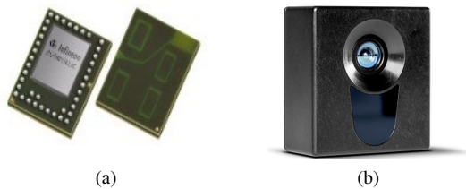
Fig. 1: (a) 60 GHz radar sensor module (Project Soli website, 2019) [32]. (b) CamBoard pico Monstar [31]
