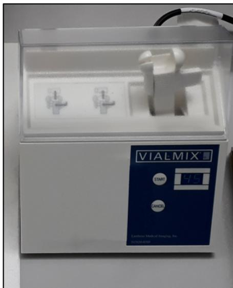
**Figure 4.9: Photograph of mixing device Vialmix for preparation of Luminity contrast agent.** Before administration, Luminity contrast agent must be activated with the mechanical shaking device. The vial is clamped into the carrier and then agitated at high frequency for 45 s.
