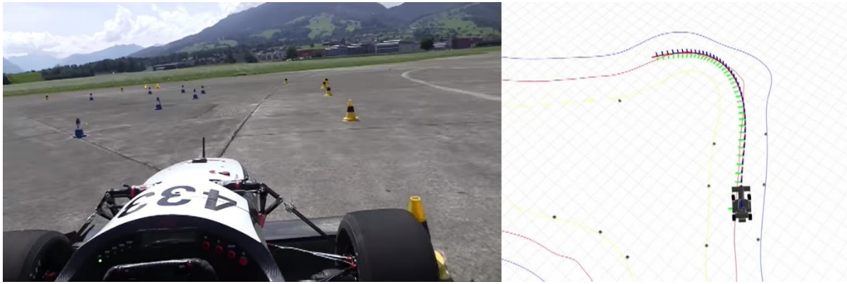
Figure 1-3: Visualization of the NMPC of the Formula Student team of the ETH Zurich, AMZ[22]
