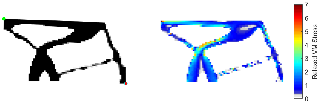
(b) Displacement figure and stress distribution for \sigma^* = 5 \text{ N/mm}^2 : \Phi = 1.88 \cdot 10^{-2} \text{ mm}^2 , \tilde{\sigma}_{PN,max} = 4.96 \text{ N/mm}^2
