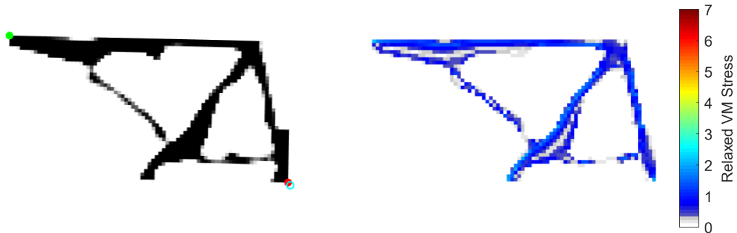
(c) Displacement figure and stress distribution for \sigma^* = 2 \text{ N/mm}^2 : \Phi = 3.71 \text{ mm}^2 , \tilde{\sigma}_{PN,max} = 2 \text{ N/mm}^2
