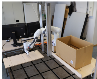
(a) The robot picks objects out of a box and places them through a simulated light barrier onto a drop area.
