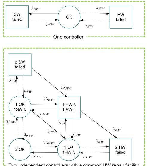
Two independent controllers with a common HW repair facility
