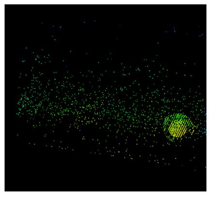
Figure 3.35.: The point cloud representing a road segment with intensities only in range 28400 to 29200. A manhole visible on the right
