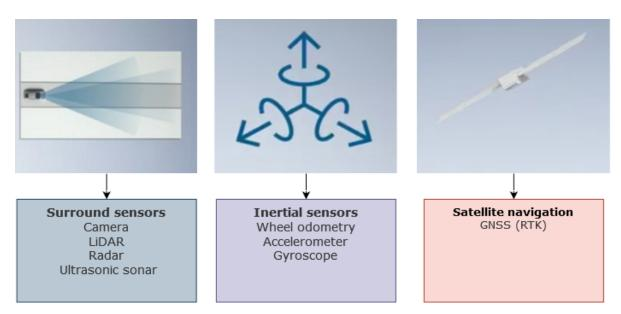
Figure 2.4.: Types of sensors used in an automated car [DPCcars, 2018; Wysocki, 2019]
