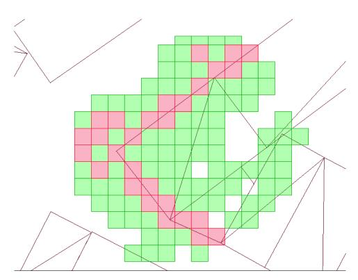
Figure 3.14.: 2D vector tiles depicting the rejected and accepted patches of point cloud subsets per one randomly selected building. Red tiles depict dense regions of a point cloud and green patches mark rejected and thus sparse point cloud areas. Buildings marked by dark edges
