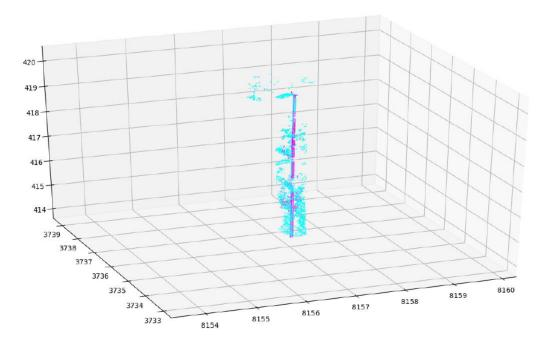
Figure 2.16.: RANSAC algorithm and detection of street lamp poles. Inliers (purple) and outliers (blue) [Wysocki & Albrecht, 2019]
