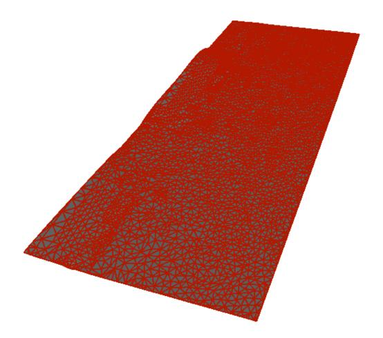
Figure 4.5.: A reconstructed road at octree level 12. Reconstructed surface consist of 6476 faces
