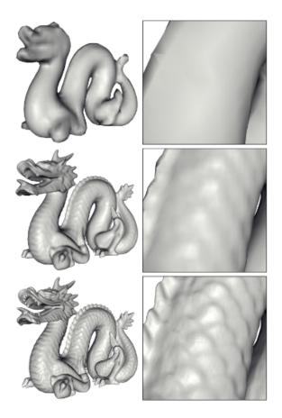
Figure 3.24.: Reconstructions of a dragon model at different octree depths 6 (top), 8 (middle), and 10 (bottom) [Kazhdan, Bolitho, & Hoppe, 2006]
