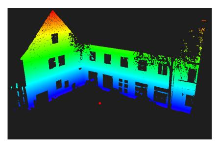
Figure 3.21.: The centre of a local coordinate system for a building. View from inside of the object. The red point indicates the local reference system origin
