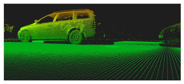
Figure 3.8.: Erroneous ALS point cloud filtered out in the Ground Points Filtering step. Those points are classified as *ground points* in a raw classification
