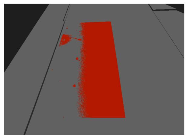
Figure 4.2.: A refined road surface (red-coloured) compared to a raw HD Map geometry. The superelevation of the road is well depicted while this information is missing in a provided HD Map test dataset
