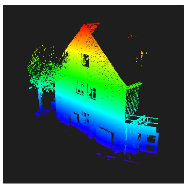
Figure 3.18.: A subset of point cloud depicting one of the building's walls before applying the RANSAC algorithm
