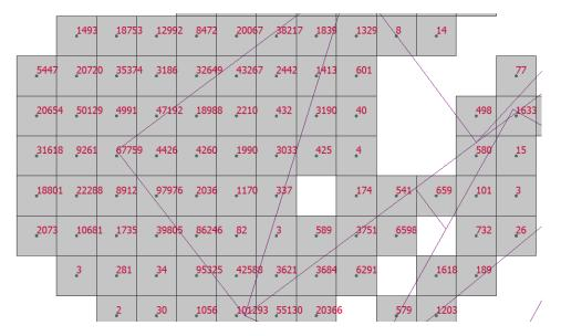
Figure 3.13.: 2D vector tiles depicting the density of point cloud subsets (grey-coloured rectangles with sum of points) per one randomly selected building
