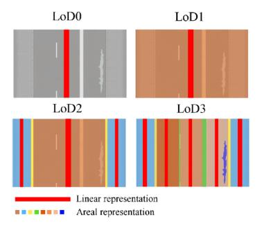
Figure 2.11.: A proposed representation of a road in the CityGML standard [Beil & Kolbe, 2017]
