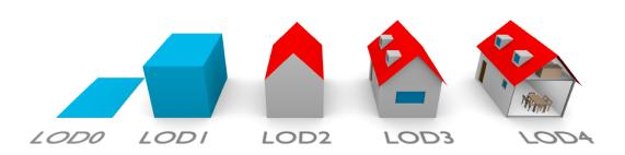
Figure 2.9.: Different Levels of Details in the CityGML standard [Biljecki, Stoter, Ledoux, et al., 2015]
