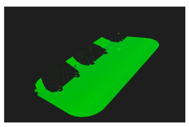
Figure 3.6.: Point cloud (ALS & MLS) cut to an area of interests of a road segment, after the Ground Points Filtering
