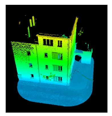
Figure 3.3.: The portion of point cloud cut by custom 3D buffer for a LoD1 building
