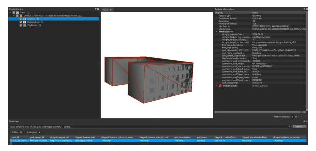
Figure 4.24.: An exported building in the FME Inspector tool. All raw semantic information kept and geometry preserved. The refined wall visible in the foreground
