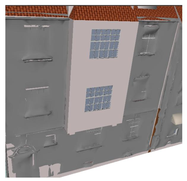
Figure 4.11.: A comparison of a reconstructed wall (dark grey colour) with an LoD3 building model (white, pink, blue colours and textures). The extruded wall modelled in an LoD3 by an operator is visible
