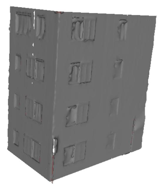
Figure 4.15.: A reconstructed building at octree level 10, 16 980 faces
