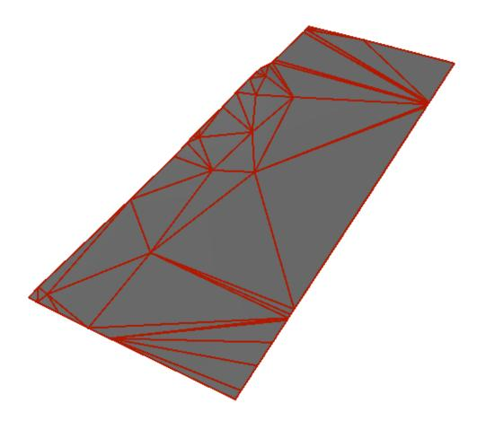
Figure 4.3.: A reconstructed road at octree level 8. Reconstructed surface consist of 36 faces
