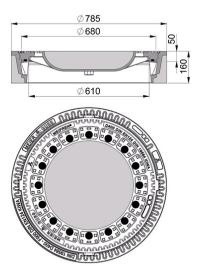
Figure 3.32.: The size of a manhole cover typical for German roads [Kemmler Baustoffe GmbH, 2020]
