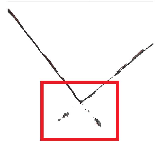
Figure 4.13.: A 2D view of reconstructed building's walls. Visible small parts reconstructed as buildings parts (within red rectangle) which in the reality describe tree branches
