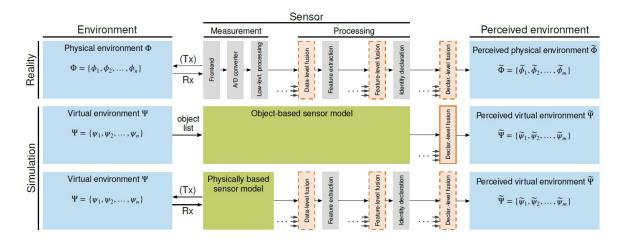
Figure 2.5.: Sensor based simulations [Schwab & Kolbe, 2019]
