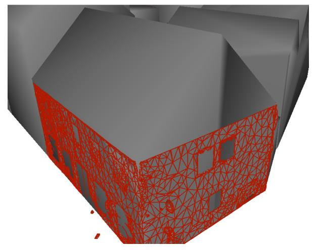
Figure 4.8.: A comparison of a reconstructed wall (red-coloured) with an LoD2 building model
