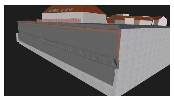
Figure 4.10.: A comparison of a reconstructed wall (dark grey colour) with an LoD3 building model
