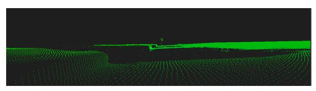
Figure 3.7.: One of *holes* in a MLS point cloud filled in with ALS points with a rectified height
