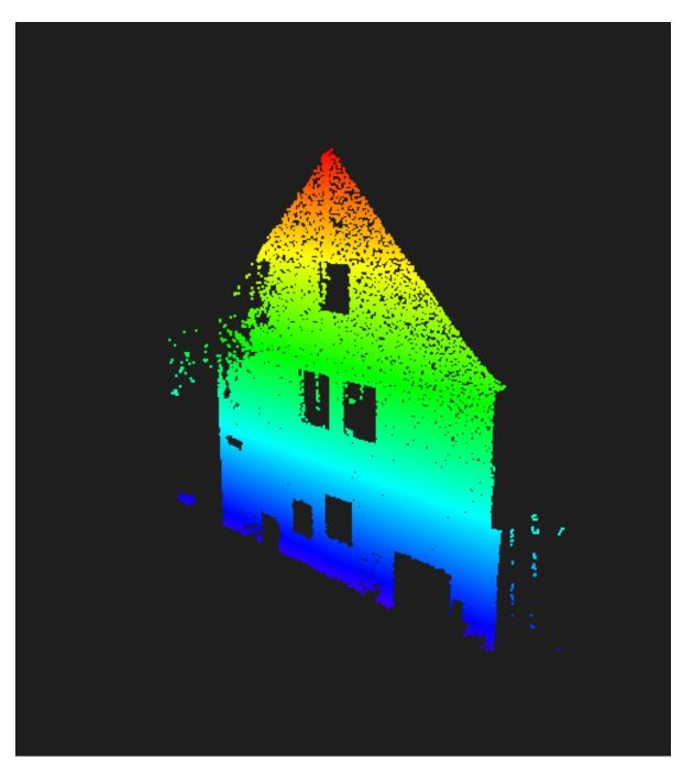
Figure 3.19.: A subset of point cloud depicting one of the building's walls after applying the RANSAC algorithm
