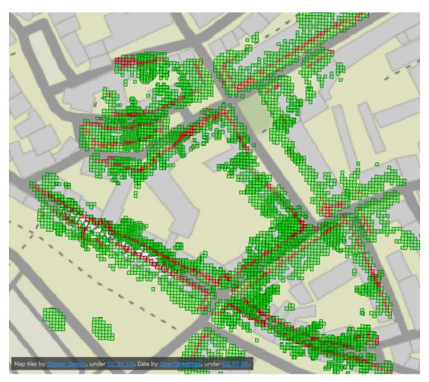
Figure 3.12.: 2D vector tiles depicting the density of point cloud subsets per buildings' group. Red tiles depict dense regions of a point cloud and green patches mark rejected and thus sparse point cloud areas
