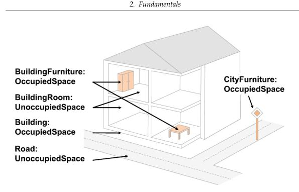
Figure 2.14.: Occupied and unoccupied space in the revised CityGML 3.0 standard [Kutzner, Chaturvedi, & Kolbe, 2020]
