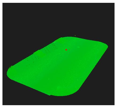
Figure 3.20.: The centre of a local coordinate system for a road segment. Red point indicates origin which is located 10 m above the data set
