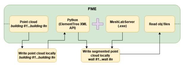
Figure 3.23.: An overview of the MeshLabServer integration within FME environment
