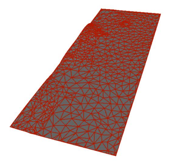
Figure 4.4.: A reconstructed road at octree level 10. Reconstructed surface consist of 1262 faces
