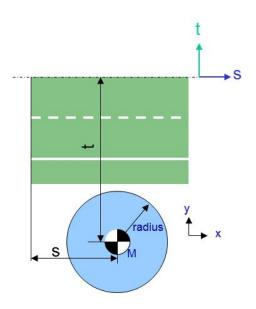
Figure 2.6.: The linear referencing in OpenDRIVE 1.6, example represents tree location definition. Each object is related to a road axis and therefore its position can be globally localized through localization of road axis [VIRES Simulationstechnologie GmbH, 2019] The XML instance can inherit various road space items like [VIRES Simulationstechnologie GmbH, 2019]:
