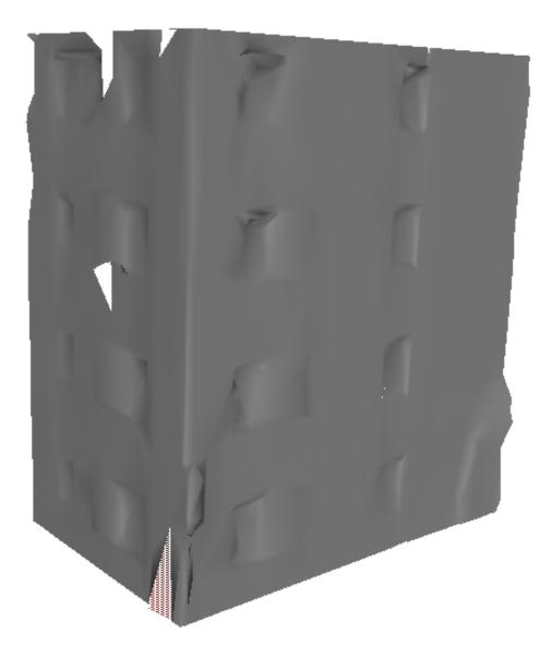
Figure 4.14.: A reconstructed building at octree level 8, 968 faces
