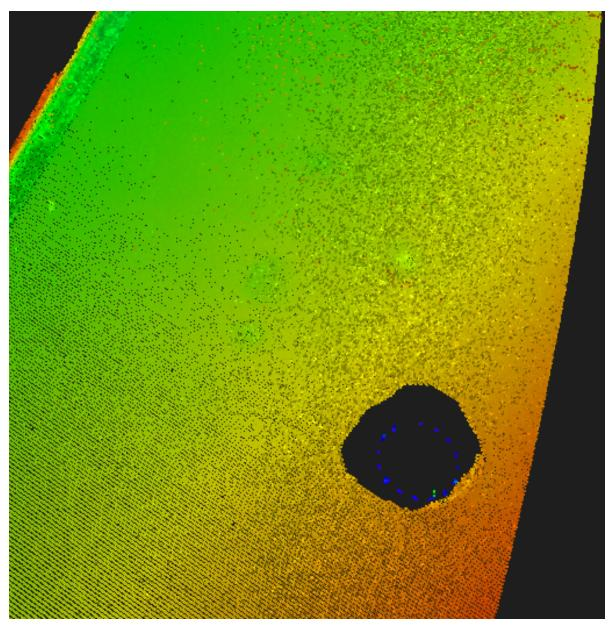
Figure 3.9.: The gap in dataset after a ground points filtering. Blue points classified incorrectly as a ground surface
