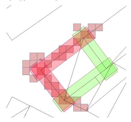
Figure 3.15.: Walls for further processing. Qualified walls marked red while rejected green. Tiles marking dense regions are red-coloured. Buildings marked by dark edges
