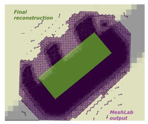
Figure 3.25.: The reconstructed mesh (purple-coloured) cut to the raw area of a reconstructed object (green-coloured) in 2D view
