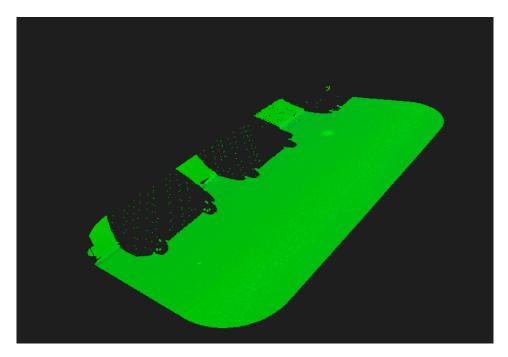
Figure 4.1.: Missing parts of an MLS dataset filled in with a sparse ALS point cloud
