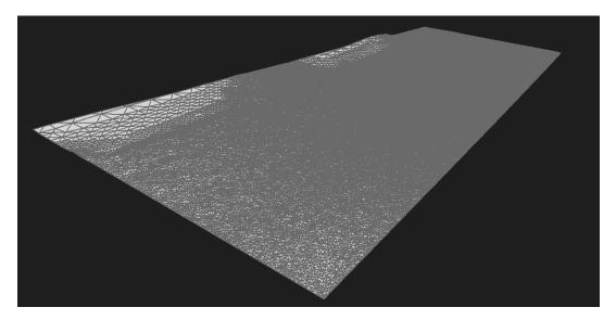
Figure 3.26.: Reconstructed mesh cut to the raw area of a reconstructed object in 3D view. 10% of simplification is applied and octree depth is set to 14
