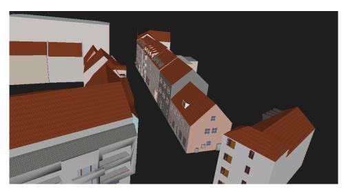
Figure 2.23.: Manually modeled LoD3 buildings
