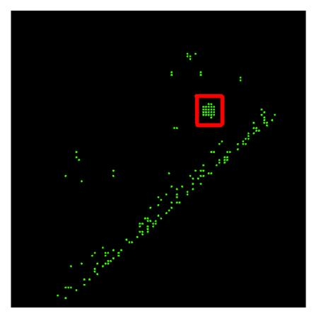
Figure 3.36.: An example of a road segment with a visible high density area (marked by red rectangle) where a manhole is located
