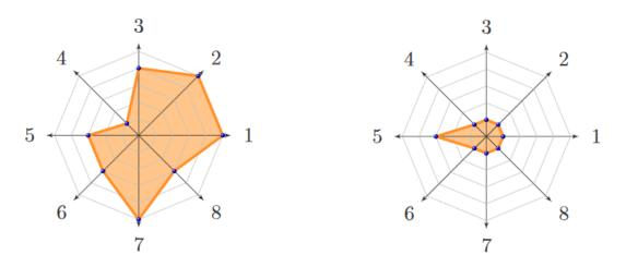
Figure 2.2.: Spider charts representing measures of scenarios complexity. Road in urban area, with signposted crossroads (left) and highway with little traffic (right). 1-lack of transparency, 2-vehicle own momentum, 3-interconnectedness, 4-novelty, 5number of conditions per element 6-number of actors, 7-openness of the target situation, 8-polytely [Schuldt, 2017]
