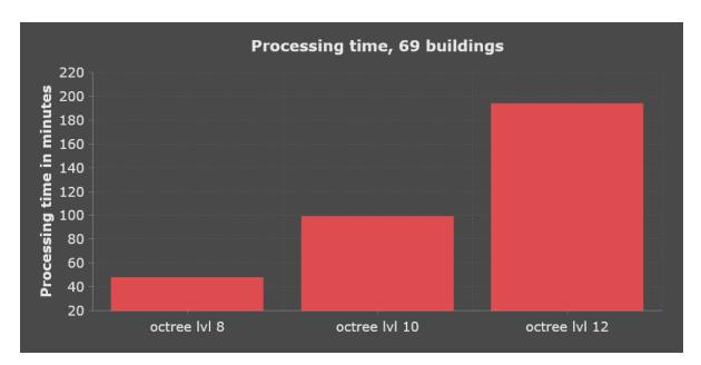
Figure 4.19.: Processing time at different octree levels for buildings. 69 Buildings refined with total 87 within a city model
