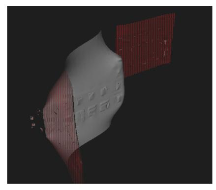
Figure 3.22.: An orientation of reconstructed surfaces. The front orientation (grey surfaces) and the back orientation (red dots). Now, simple swap allows to orient faces towards the desired, outward direction
