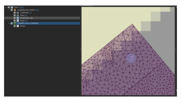
Figure 3.40.: Road, Hole, and HoleSurface as one CityGML 3.0 model
