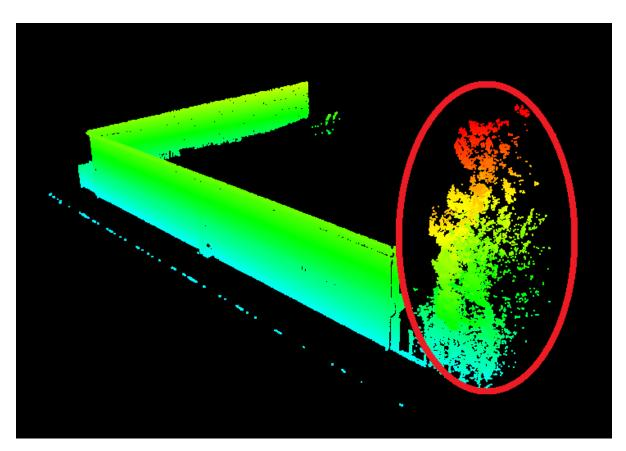
Figure 3.11.: Point cloud (MLS) cut to an area of interests of a building, after the Ground Points Filtering. The red circle indicates one of the outliers portion, a point cloud depicting tree
