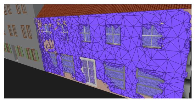
Figure 4.9.: A comparison of a reconstructed wall (blue-coloured) with features of an LoD3 building model
