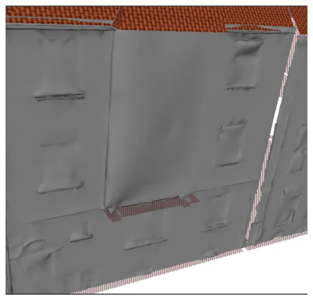
Figure 4.12.: A reconstructed wall's extrusion within a wall (dark grey colour) and a roof of LoD3 building model (textures). A visible slight wall's extension in the place of the extrusion
