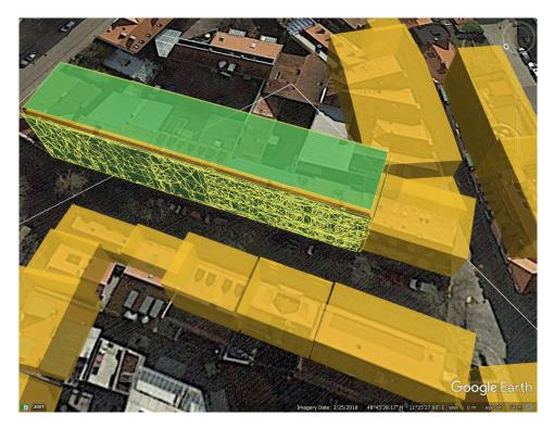
Figure 4.25.: The exported buildings in Google Earth Pro. The green highlight shows a picked object and its refined structure (yellow edges)
