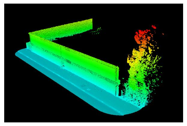
Figure 3.10.: Point cloud (MLS) cut to an area of interests of a building, before the Ground Points Filtering
