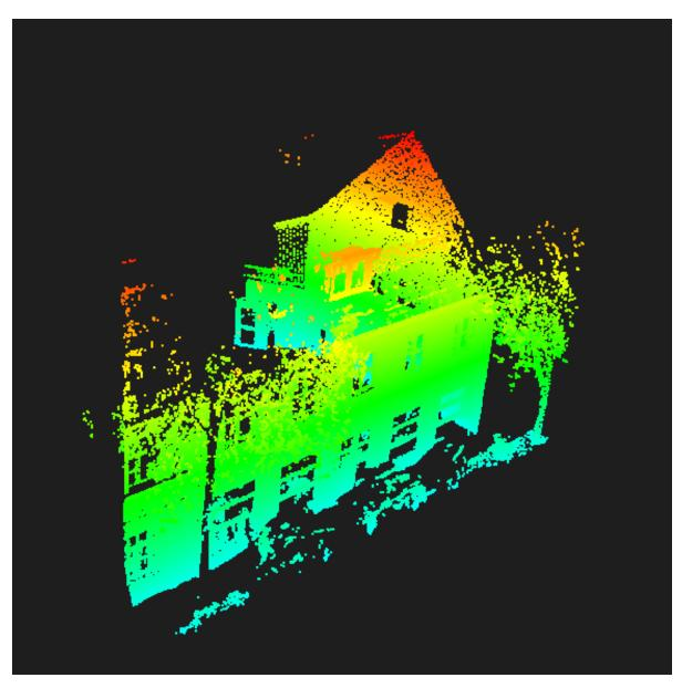
Figure 3.16.: A point cloud subset representing a building after selection of valid walls. Ground points already rejected and boundaries of walls' buffers visible. Outliers still present in the subset (e.g. trees, cars at the parking space)
