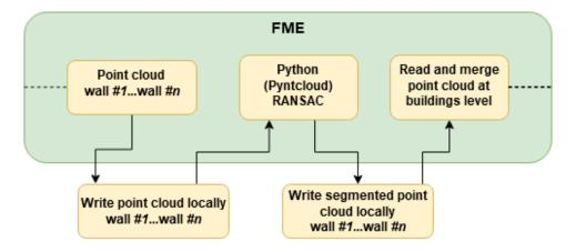
Figure 3.17.: An overview of the pyntcloud and RANSAC integration FME environment
