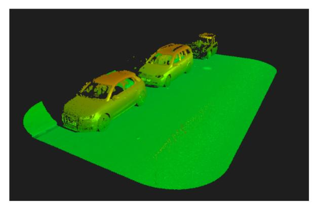
Figure 3.5.: Point cloud (ALS & MLS) cut to an area of interests of a road segment, before the Ground Points Filtering
