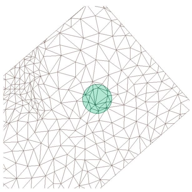
Figure 3.39.: A refined geometry of a road segment (white polygons) and a cut out geometry of a manhole (green polygons)
