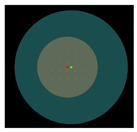
Figure 3.38.: A searching area of a manhole's exact centre. The first point of interest is marked by the green point, first buffer is marked with blue colour. The final centre point (red colour) is a gravity centre of patches within the second buffer (orange colour)
