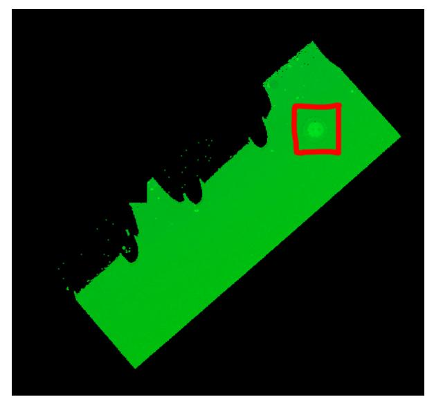
Figure 3.34.: An example of a point cloud depicting a road segment with a visible manhole, area marked by the red rectangle. The Ground Points Filtering method applied to filter out irrelevant points
