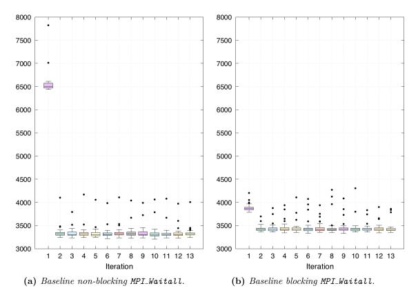
**Figure 4.5:** Boxplots showing stability of the iterations on NVidia testbed. Y axis presents times per iteration in µs. The first iteration takes longer, and is a lot less stable.
