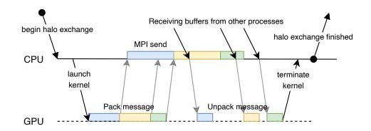
**Figure 3.13:** Splitting buffer to multiple chunks to enable pipelining of packing, MPI communication, and unpacking in case the packing functions take the same time to finish for all blocks.
