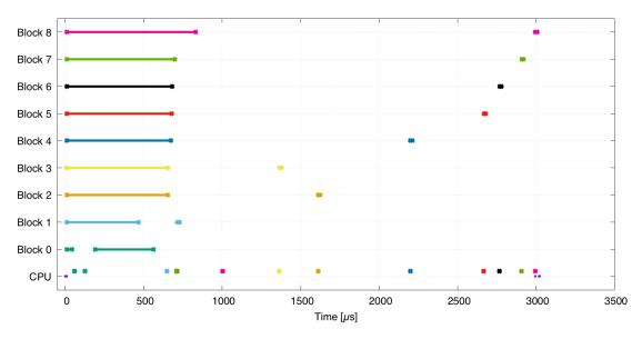
**Figure 4.8:** One iteration of taskqueue non-blocking with per-block channel. The CPU processes events regarding all blocks – an event is a dot of respective block's colour.
