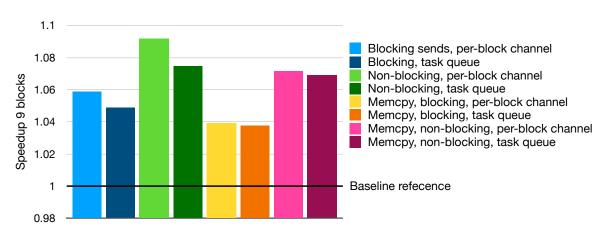
**Figure 4.7:** Taskqueue implementations speedup on NVidia. Fastest baseline is set as reference, the speedups of taskqueue approaches ranges from ca. 4 to 9 %.
