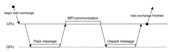
**Figure 2.5:** General workflow of the halo exchange. First, the GPU packs the message to send in send buffer. Next, the CPU communicates over MPI. Once the communication finishes, the GPU can unpack the message in recv buffer.
