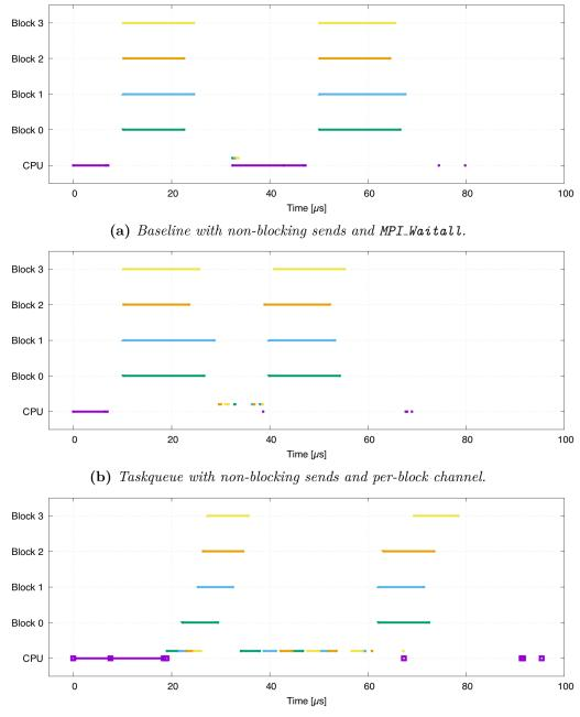
(c) Taksqueue with memcpy, non-blocking sends, and per-block channel.
