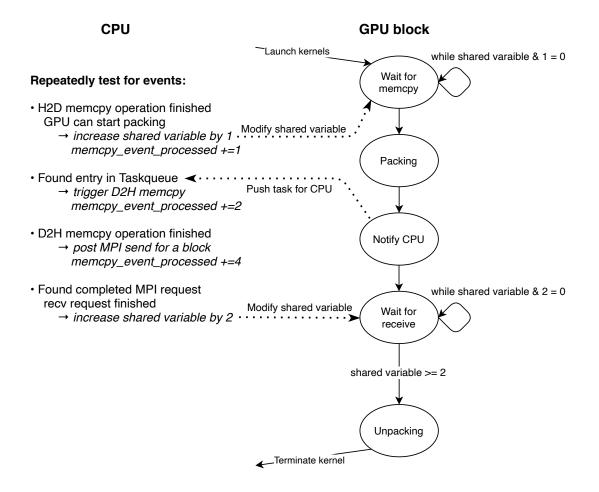
Figure 3.11: FSM of one halo exchange iteration and one GPU block for memcpy variant.
