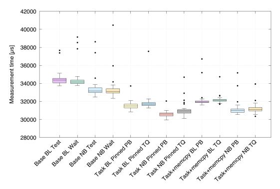
Figure 4.11: Boxplot with summary over times of all measurements on NVidia with 9 blocks. Apart from some outliers, the stability of the results is good. (Base=baseline, Task=taskqueue, BL=blocking sends, NB=non-blocking sends, Test=MPI\_Testany, Wait=Test=MPI\_Waitall, PB=per-block channel, TQ=task queue)
