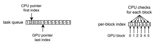
(a) Single task queue approach. GPU blocks enqueue at the bottom and CPU dequeues from the front.
