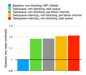
Figure 4.17: Speedup of selected implementations on NVidia with very large workloads. The baseline is set as reference, and the speedups of taskqueue approaches range from 1.18 to 1.21 This is the only workload where memcpy outperforms pinned host memory taskqueue.
