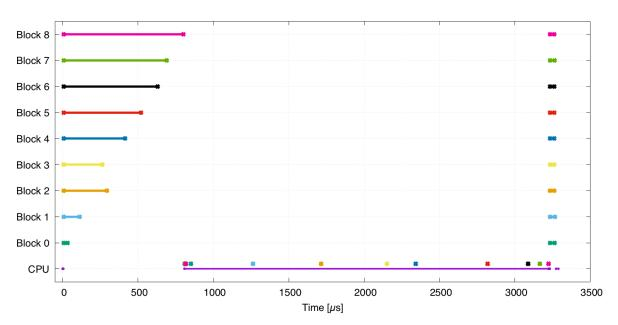
**Figure 4.4:** One iteration of non-blocking baseline with MPI\_Testany on NVidia. The 'Block' lines denote packing and unpacking times. The violet 'CPU' line denotes the communication phase, the dots of respective colours denote receiving a message of a particular block.
