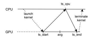
Figure 4.2: Communication scheme in the ping-pong CPU-GPU roundtrip implementation.
