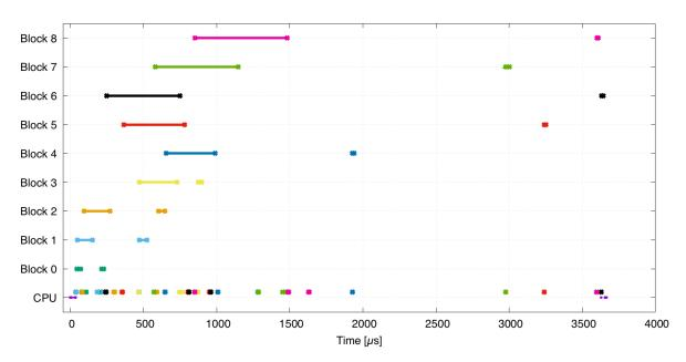
**Figure 4.10:** One iteration of taskqueue memcpy non-blocking with per-block channel on NVidia. The packing starts first when the buffer is copied over, and there is twice as many events in the system.
