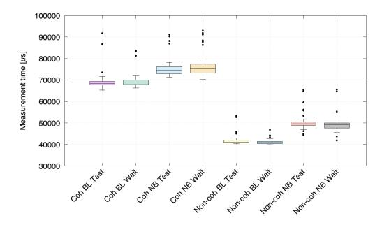
Figure 4.27: Boxplot with summary over measured times of baseline coherent and non-coherent experiments on AMD with 9 blocks. The non-blocking versions have more outliers and the stability of the results is lower, but overall, the results are reliable. (Coh=coherent, Non-coh=non-coherent, BL=blocking sends, NB=non-blocking sends, Test=MPI\_Testany, Wait=Test=MPI\_Waitall)
