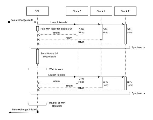
**Figure 3.3:** Workflow of one baseline iteration. The halo exchange starts with launching GPU kernels for packing. The CPU waits for all kernels to finish this operation, and after that all communication takes place. When that is done, the unpacking kernels are launched and finally, the iteration can finish after all tasks were completed.
