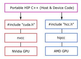
Figure 2.3: Compiling HIP code for AMD and NVidia devices. [7]
