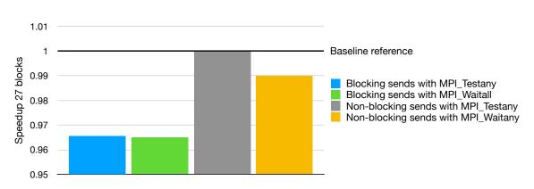
**Figure 4.6:** Baseline implementations with 27 blocks – speedup on NVidia. Non-blocking communication still outperforms the blocking one.
