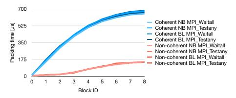
**Figure 4.25:** AMD baseline packing times with 9 blocks. Red lines represent non-coherent memory options, blue lines the coherent ones. (BL=blocking sends, NB=non-blocking sends)
