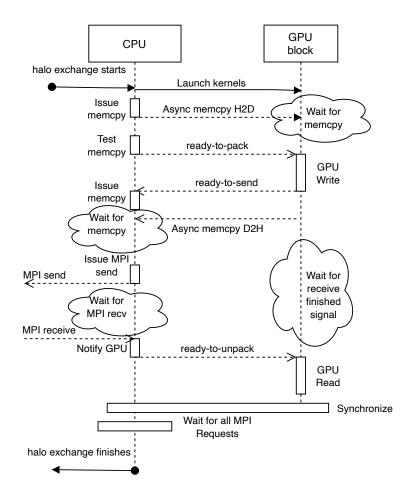
Figure 3.10: Interactions between the CPU and a GPU block in one iteration.
