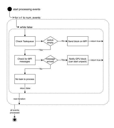
Figure 3.8: Workflow of a CPU processing events in the Taskqueue approach.
