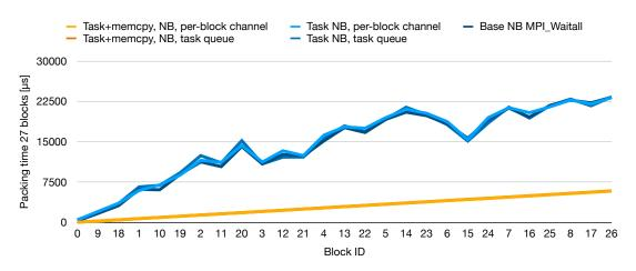
**Figure 4.19:** NVidia packing times with very large workload. Orange lines represent taskqueue memcpy options, blue lines baseline and taskqueue pinned host memory options. (Base=baseline, Task=taskqueue, NB=non-blocking sends)
