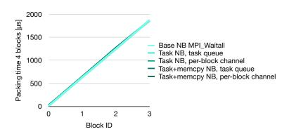
**Figure 4.14:** NVidia packing times with 4 blocks and 16 threads per block. All tested options yielded very similar behavious. Comparatively longer times to previous plots are due to only 16 packing threads per block. (Base=baseline, Task=taskqueue, BL=blocking sends, NB=non-blocking sends)
