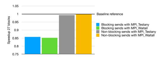
**Figure 4.23:** Coherent baseline implementations speedup on AMD with 27 blocks. Unlike in fig. 4.20 with 9 blocks, non-blocking communication outperforms the blocking one. The difference is approx. 15 %.
