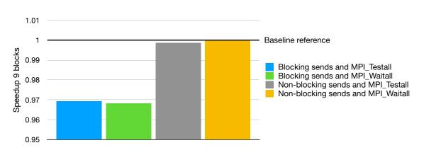
**Figure 4.3:** Baseline implementations speedup on NVidia. Non-blocking communication outperforms the blocking one.
