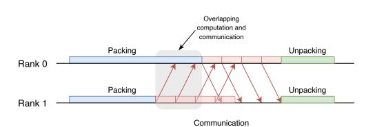
(a) Baseline workflow with overlapping blocking communication and computation. Rank 1's packing finishes sooner and therefore rank 0 experiences overlapping of communication (non-blocking receive operations) and computation. However, then, even if all recv buffers are available, it unpacking must wait for blocking send operations to return.
