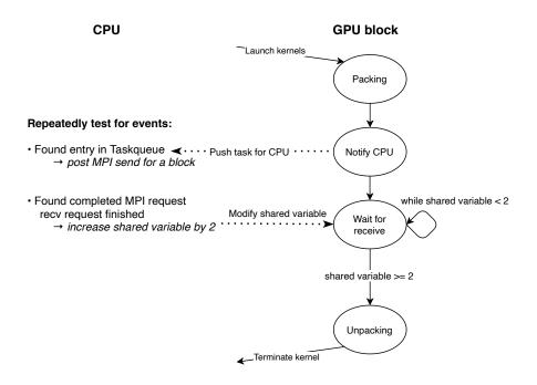
Figure 3.7: FSM of one halo exchange iteration and one GPU block.
