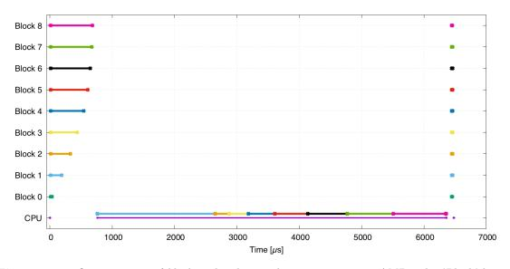
Figure 4.22: One iteration of blocking baseline with MPI\_Testany on AMD. The 'Block' lines denote packing and unpacking times. The lines of respective colours denote time of blocking send operations for the respective blocks. Block 1's send operation is disproportionally long.
