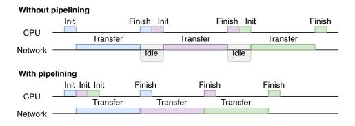
**Figure 3.5:** Comparison of sequential and pipelining approaches to network communication. Pipelining enables better utilization of the network, which is the critical resource.
