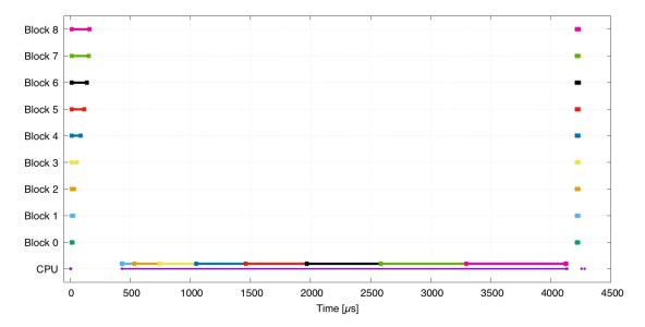
Figure 4.26: One iteration of non-coherent blocking baseline with MPI\_Testany on AMD. The 'Block' lines denote packing and unpacking times. The lines of respective colours denote time of blocking send operations for the respective blocks. Unlike in fig. 4.22 with coherent buffers, Block 1's send operation is proportional to others.
