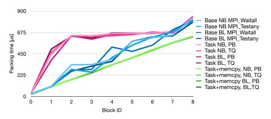
**Figure 4.9:** NVidia packing times with 9 blocks. Green lines represent taskqueue memcpy options, purple lines taskqueue pinned host memory options, and blue lines baseline. (Base=baseline, Task=taskqueue, BL=blocking sends, NB=non-blocking sends, PB=per-block channel, TQ=task queue)
