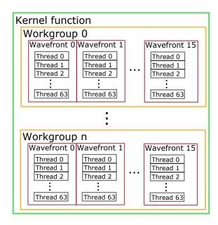
Figure 2.1: Parallelization divisions in a GPU kernel function.
