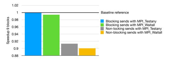
**Figure 4.20:** Coherent baseline implementations speedup on AMD with 9 blocks. Blocking communication outperforms the non-blocking one by approx. 9 %.
