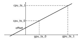
Figure 4.1: Finding conversion function from GPU timestamps to CPU timestamps. If there are 2 points in time where both the CPU and GPU timestamp values are known, the linear conversion function for an arbitrary GPU timestamp can be calculated.
