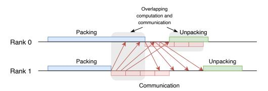
(b) Baseline workflow with overlapping non-blocking communication and computation. Rank 1's packing finishes sooner and therefore rank 0 experiences overlapping of communication (nonblocking receive operations) and computation. As non-blocking sends are posted, rank 0 can begin unpacking while its send operations are still on the way. Nontheless, rank 1's unpacking must wait for the data to arrive.
