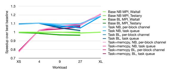
**Figure 4.28:** Speedup over all workloads on NVidia. The workload size is ascending. Green lines represent baseline, blue ones taskqueue with pinned host memory, and purple ones taskqueue with memory. (Base=baseline, Task=taskqueue, BL=blocking sends, NB=non-blocking sends)
