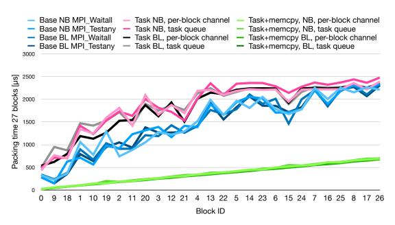
**Figure 4.13:** NVidia packing times with 27 blocks. Green lines represent taskqueue memcpy options, purple and grey lines taskqueue pinned host memory options, and blue lines baseline. (Base=baseline, Task=taskqueue, BL=blocking sends, NB=non-blocking sends)
