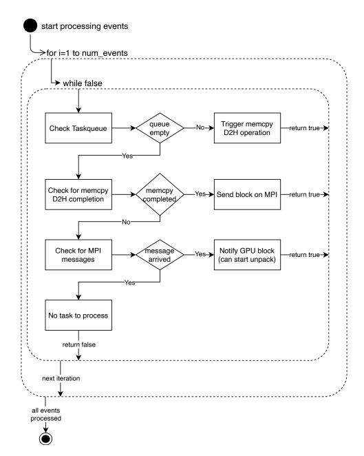
Figure 3.12: Workflow of a CPU processing events in the Taskqueue memcpy approach.
