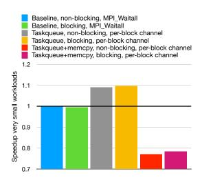
**Figure 4.16:** Speedup of selected implementations on NVidia with very small workloads. Faster baseline is set as reference, the speedups of pinned host memory taskqueue approaches are around 1.09, while memcpy options range between 0.77 and 0.79
