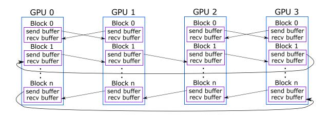
**Figure 2.6:** An example communication scheme. Block x always communicates with block x of another GPU. In this example, block 0 exchanges data pairwise – with preceding and succeeding GPU, respectively, data of block 1 is sent to the succeeding GPU and data of block n is sent to preceding GPU.
