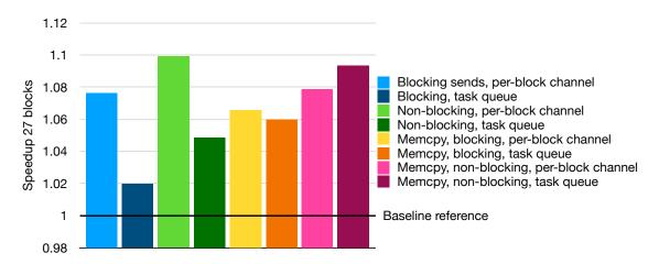
**Figure 4.12:** Taskqueue implementations speedup on NVidia with 27 blocks. Fastest baseline is set as reference, the speedups of taskqueue approaches ranges from ca. 2 to 10 %.
