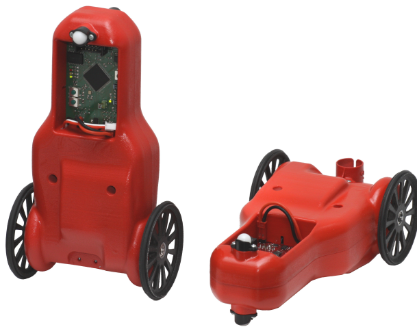
Figure 1.1: The TWIP developed at the Chair of Automatic Control at Technical University of Munich. Although – as demonstrated on the right-hand side – it has the ability to also drive in a horizontal position, the aim of this work will be to stabilize it in its upright position as pictured on the left-hand side.
