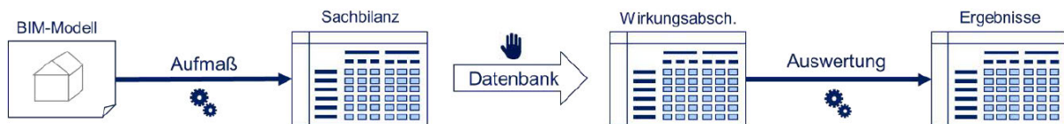
Figure 2-14: Procedure for semi-automated, BIM-based EE calculation (Forth 2018)
