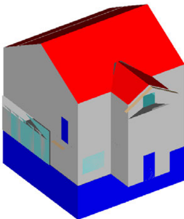
Figure 3-12: Result of automated generation of 2 nd Level SB in Revit using fully automated export functionality
