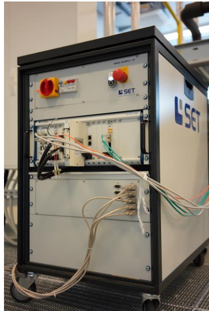
6 embedded controllers to acquire the signals
