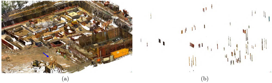
Figure 4.9: Crane ROIs in point cloud: (a) original point cloud with a blue arrow indicating the location of the crane; (b) Crane ROIs, notice the presence of other thin and tall objects additional to the cranes. Test dataset: Nr. 1.
