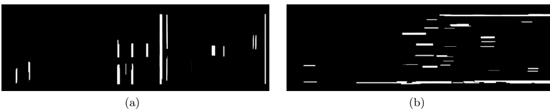
Figure 4.16: Horizontal and vertical formwork blobs: (a) vertical formwork blobs; (b) horizontal formwork blobs in dataset Nr. 3.
