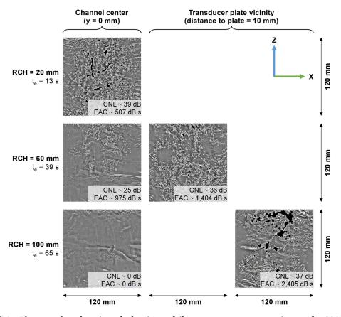
**Figure 6.4:** Photographs of sonicated aluminum foils at a constant energy input of ~ 200 kJ/kg<sub>TS</sub> at different locations within the reactor (centrally positioned and positioned 10 mm apart from the transducer plate) for three different reaction chamber heights (RCHs). For RCH = 20 mm, the two locations are identical. Cavitation noise levels (CNLs), exposure times ( $t_e$ ) and exposition indices (EAC = CNL·t<sub>e</sub>) are shown next to the photographs.
