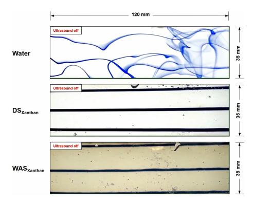
**Figure C.2:** Visualization of the flow behavior of water,  $DS_{Xanthan}$  and  $WAS_{Xanthan}$  in an ultrasound flatbed reactor before and during treatment by the use of dye streams. Video is available at https://doi.org/10.1016/j.ultsonch.2019.01.024.
