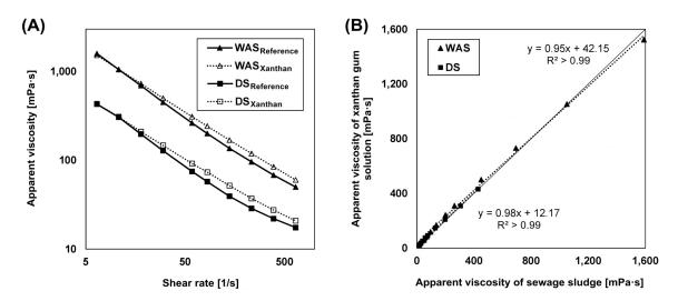
**Figure 5.2:** Relationship between shear rate and apparent viscosity for  $WAS_{Reference}$ ,  $WAS_{Xanthan}$ ,  $DS_{Reference}$ , and  $DS_{Xanthan}$  in logarithmic scale (A), and linear regressions for the fit between sludges and xanthan solutions (B).
