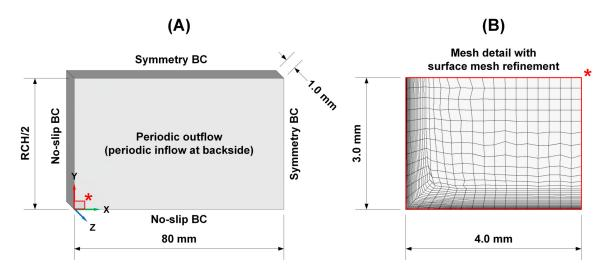
**Figure D.2:** 3-D periodic fluid domain and applied boundary conditions (BCs, subfigure A) and detail of the final mesh showing hexahedron elements and surface mesh refinements at the no-slip walls (subfigure B), for a reaction chamber height (RCH) of 100 mm. The location of the mesh cutout within the domain is marked by a red frame in subfigure (A).
