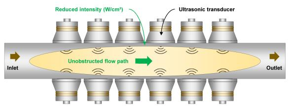
Figure 2.3: Schematic of a tube-shaped flat transducer reactor.
