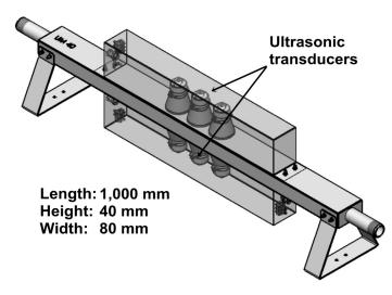
Figure 4.1: Schematic of the novel ultrasonic flatbed reactor.
