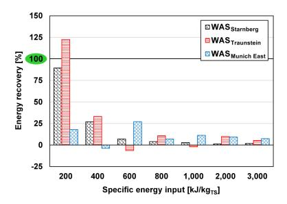
**Figure 4.6:** Energy recovery, i.e., ratio of electrically invested energy and regained energy by additional methane vs. specific energy input. 100% denote an energy- neutral operation.
