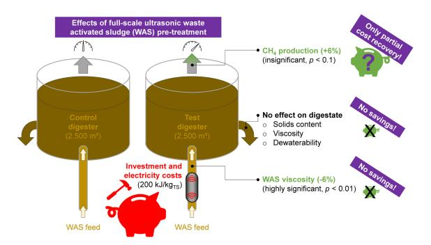
**Figure E.1:** Graphical abstract Paper IV (Full-scale assessment of ultrasonic sewage sludge pre-treatment using a novel double-tube reactor).
