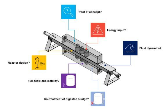
Figure 3.1: 3-D schematic of the novel ultrasonic flatbed reactor and key research topics along with graphical identifiers.
