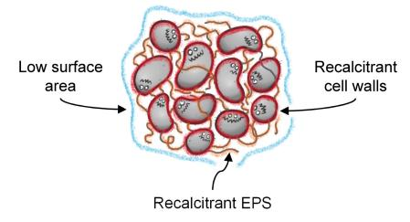
**Figure 1.2:** Illustration of a waste activated sludge floc and its recalcitrant properties, with EPS = extracellular polymeric substances.
