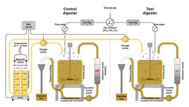
**Figure 8.1:** Schematic of the laboratory digester system, including feeding system, anaerobic digesters (control and test digester), recirculation loops, ultrasonic reactors, and gas analysis system.
