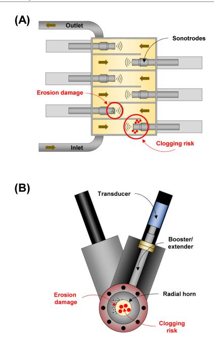
**Figure 2.2:** 2-D schematics of a conventional sonotrode reactor (A, side view) and a radial horn reactor (B, front view), showing areas of increased clogging risk and erosion damage.
