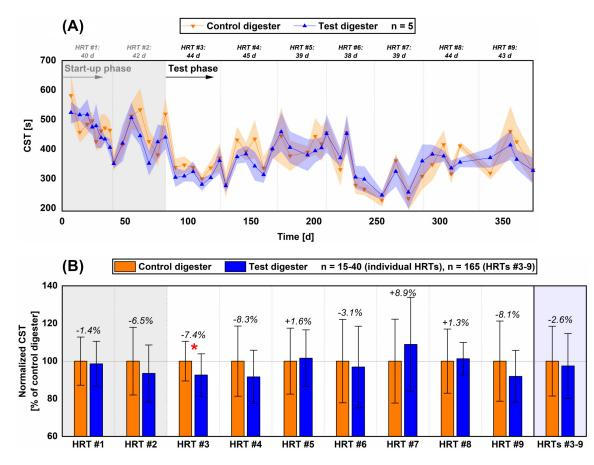
**Figure 7.5:** Development of the capillary suction time (CST) of the digestate from the control and the test digester (A) and normalized CST relative to the control digester (B). Significant differences between two data sets are denoted with an asterisk. Error bands and error bars denote the standard deviation of the mean.
