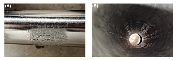
**Figure 10.2:** Erosion damage on the inner (A) and on the outer transducer surfaces (B) of the full-scale ultrasound reactor employed at the Starnberg wastewater treatment plant.
