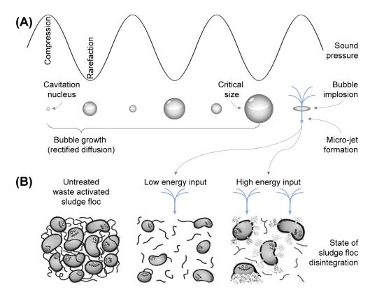
**Figure 2.1:** Principle of rectified mass diffusion (subfigure A) and different stages of sludge disintegration (subfigure B), including an intact sludge floc, a de-agglomerated floc after sonodispergation (low energy input treatment) and a completely disintegrated floc with severe cell lysis (high energy input treatment).
