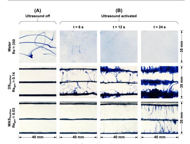
**Figure 5.3:** Photographs representing the flow conditions of water,  $DS_{Xanthan}$  and  $WAS_{Xanthan}$  before US treatment (A), and during ultrasonic irradiation at different times after treatment activation (B). The images represent the flow in the center of the cavitational field, as indicated in Figure 5.1C
