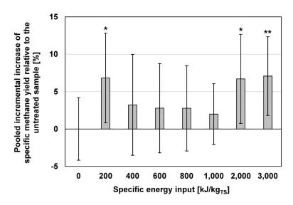
**Figure 4.5:** Pooled incremental increase of specific methane yield relative to the untreated sample vs. specific energy input. Error bars indicate standard deviation from the average of the nine values. Significant differences to the untreated sample are indicated with an asterisk at a 5% significance level and with two asterisks at a 1% significance level, according to the Student's *t* test.
