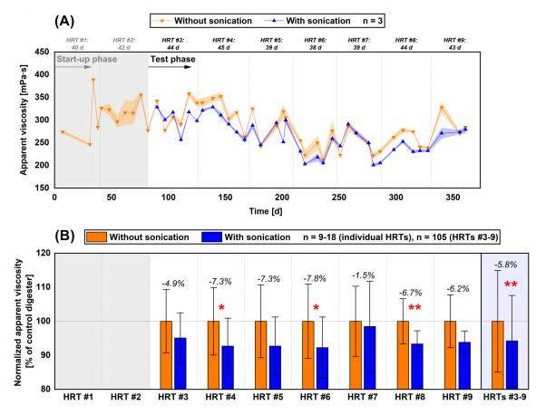
**Figure 7.2:** Development of apparent viscosity of waste activated sludge with and without sonication at a shear rate of 644 1/s (A) and normalized apparent viscosity relative to the control digester (B). Significant and highly significant differences between two data sets are denoted with one, or two asterisks, respectively. Error bands and error bars denote the standard deviation of the mean.
