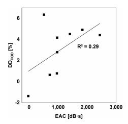
**Figure D.3:** Linear regression between exposure to acoustic cavitation (EAC, i.e., cavitation noise level multiplied by exposure time) and degree of disintegration ( $DD_{COD}$ ).
