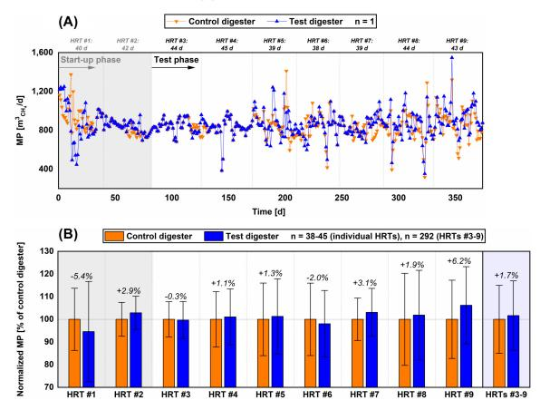
**Figure 7.3:** Development of daily methane production (MP) of the control and the test digester (A) and normalized MP relative to the control digester (B). Error bars denote the standard deviation of the mean.
