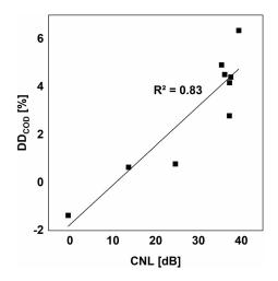
**Figure 6.6:** Linear regressions between cavitation noise level (CNL) and degree of disintegration  $(DD_{COD})$ .
