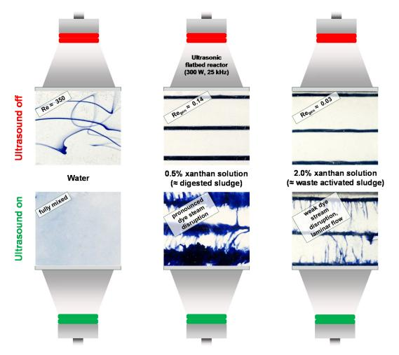
**Figure C.1:** Graphical abstract Paper II (*Impact of ultrasound-induced cavitation on the fluid dynamics of water and sewage sludge in ultrasonic flatbed reactors*).
