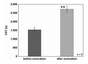
**Figure 8.4:** Capillary suction time (CST) of digested sludge before and after batch sonication at a specific energy input of 2,000 kJ/kg<sub>TS</sub>. Error bars denote the standard deviation of the mean (n = 5).
