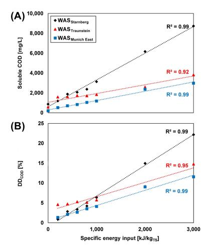
Figure 4.2: Solubilization of COD (A) and degree of disintegration DD<sub>COD</sub> (B) vs. specific energy input.
