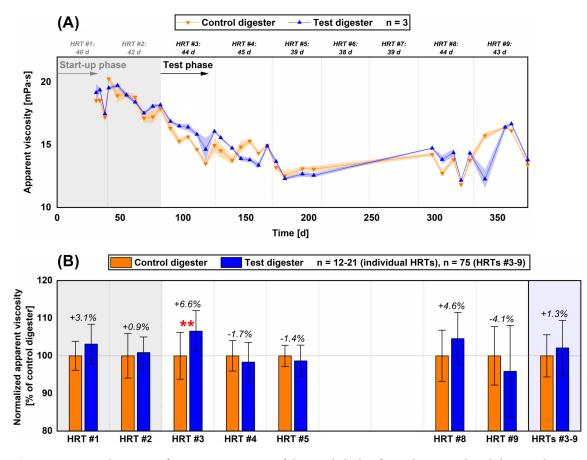
**Figure E.2:** Development of apparent viscosity of digested sludge from the control and the test digester at a shear rate of 644 1/s (A) and normalized apparent viscosity relative to the control digester (B). Highly significant differences between two data sets are denoted with two asterisks. Error bands and error bars denote the standard deviation of the mean.
