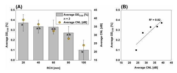
**Figure 6.9:** Average degree of disintegration ( $DD_{COD}$ ) and average cavitation noise level (CNL) for all reaction chamber heights (RCHs) tested (subfigure A) and linear regression analysis of both parameters (subfigure B). Error bars denote the standard deviation, and letters a and b indicate significance levels. Data sets without a common letter are significantly different at p < 0.05.
