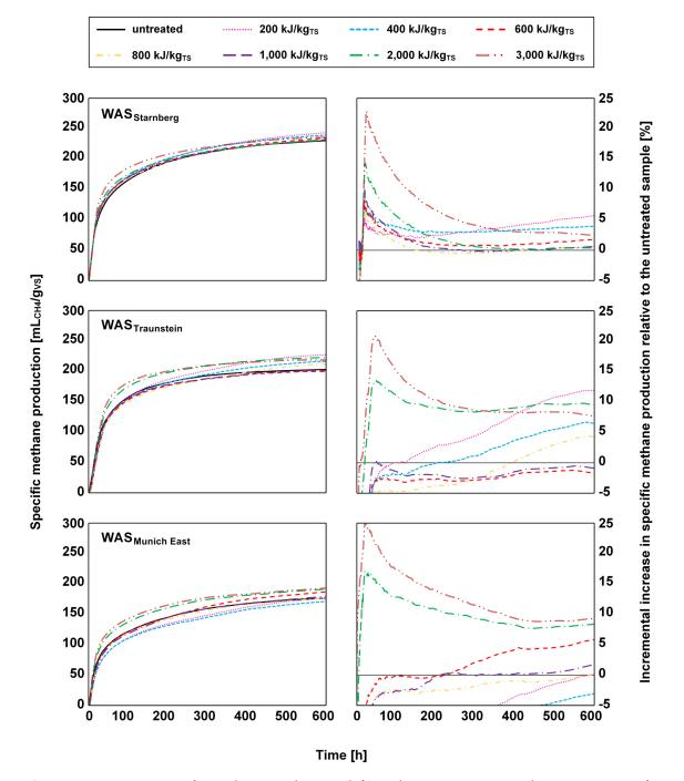
**Figure 4.4:** Average specific methane production (left) and average incremental increase in specific methane production relative to the untreated sample (right) at different specific energy inputs.
