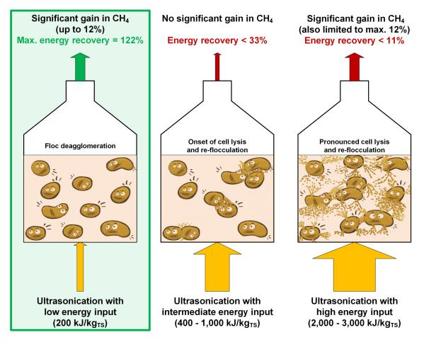
**Figure B.1:** Graphical abstract Paper I (*Energy-positive sewage sludge pre-treatment with a novel ultrasonic flatbed reactor at low energy input*).
