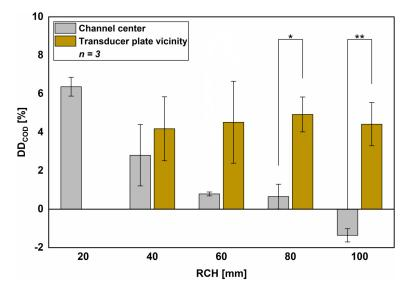
**Figure 6.5:** Degree of disintegration (DD<sub>COD</sub>) for samples taken at the channel center and in transducer plate vicinity for all tested reaction chamber heights (RCHs) at a constant energy input of ~ 200 kJ/kg<sub>TS</sub>. Error bars denote the standard deviation. Significant differences between inner and outer measurement locations are shown using asterisks (\* = significant at p < 0.05, \*\* = highly significant at p < 0.01).
