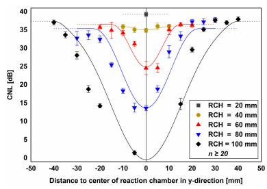
**Figure 6.3:** Distribution of cavitation noise levels (CNLs) along the  $y_0$ -axes for reaction chamber heights (RCHs) from 20 - 100 mm. Markers denote average values of  $n \ge 20$  measurements, while error bars indicate the standard deviation. Solid lines represent polynomial approximations of the measurement values based on the mirrored measurement data, whereas dotted lines represent constant linear extrapolations of the outmost measurement values.
