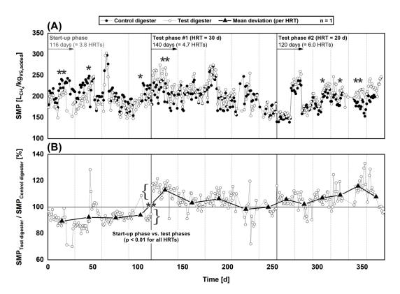
**Figure 8.2:** Development of daily specific methane production (SMP) of the control and the test digester (A) and percentage difference between both digesters (B). Significant and highly significant differences between the two data sets are denoted with one or two asterisks, respectively, for each hydraulic retention time (HRT).
