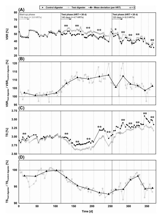
**Figure 8.3:** Development of volatile solids removal (VSR) (A) and total solids (TS) concentration of the digestate (C) of the control and the test digester, and percentage differences between both digesters (B and D). Significant and highly significant differences between the two data sets were denoted with one or two asterisks, respectively, for each hydraulic retention time (HRT). Error bands denote the standard deviation of the mean (n = 3).
