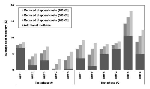
**Figure 8.6:** Estimation of average cost recoveries (i.e., ratio of electricity costs vs. cost savings due to additional methane and reduced residual sludge mass) for each HRT of both test phases.
