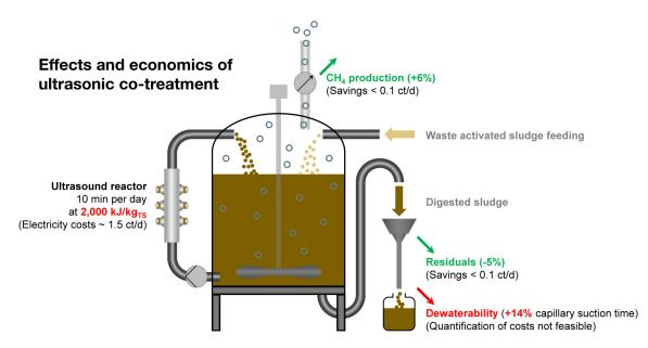
**Figure F.1:** Graphical abstract Paper V (From pre-treatment to co-treatment - How successful is ultrasonication of digested sewage sludge in continuously operated anaerobic digesters?).
