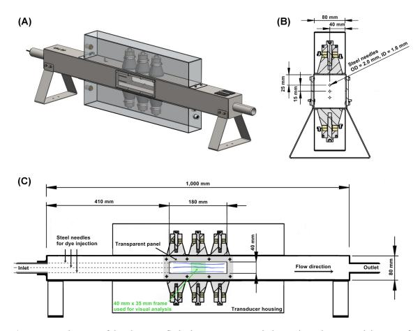
**Figure 5.1:** Schematic of the ultrasonic flatbed reactor setup, including a three-dimensional drawing of the reactor (A), a cross-sectional plot (B, where OD is outer diameter and ID is inner diameter), and a longitudinal section plot (C).
