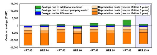
**Figure 7.6:** Development of the costs and savings of the full-scale ultrasound (US) pre-treatment, with HRT = Hydraulic retention time. \*The cost reduction due to reduced pumping energy demand (< 1  $\in$  /HRT) is too little to be discernible in the graph.
