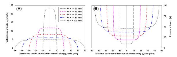
**Figure D.4:** Velocity profiles in  $u_z$ -direction (subfigure A) and affiliated exposure times  $t_e$  (subfigure B) along the  $y_0$ -axis for all tested reaction chamber heights (RCHs). For better visibility, the scale for exposure times was cut at 100 s as theoretical exposure times close to reactor walls were infinitely high due to the no-slip condition ( $u_z = 0$ ). Exposure times for the slowest 2% of the flow are therefore not shown).
