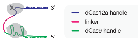
Figure 34. Single RNA that guides dCas9 and ddCas12a to their targets simultaneously (c9c12aRNA). The structure contains the RNA handles that complex with dCas9 and ddCas12a and a linker element.
