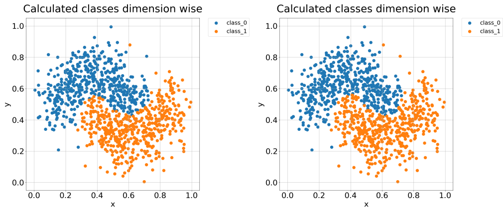
Figure 4.17: The calculated classes for the dimension-wise method. The left side is for the single class density estimation with the guided volume error measure, while the right is for the one-vs-others approach with the misclassification error measure.
