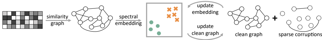
Figure 3.1: Overview of the proposed Robust Spectral Clustering (RSC) approach. Given a (similarity) graph we alternate between updating the spectral embedding based on the Laplacian of the clean graph, and updating the latent clean graph by removing sparse corruptions.
