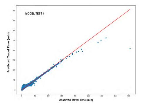
Figure 110: Convolutional Neural Network (ANN) model 4 test correlation plot
