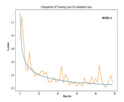
Figure 68: Convolutional Neural Network (CNN) model 4 training and validation loss curves
