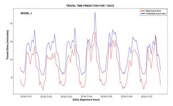
Figure 62: Artificial Neural Network (ANN) models 3 travel time prediction per hour
