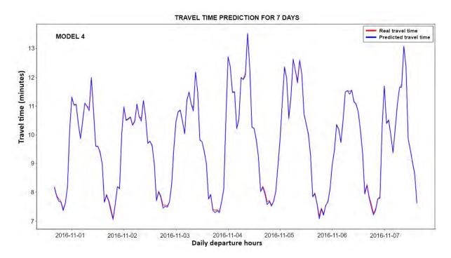
Figure 113: Artificial Neural Network (ANN) model 4 real travel time prediction per hour
