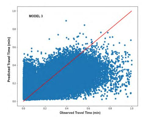
Figure 92: Long Short-Term Memory (LSTM) model 3 training and validation correlation
