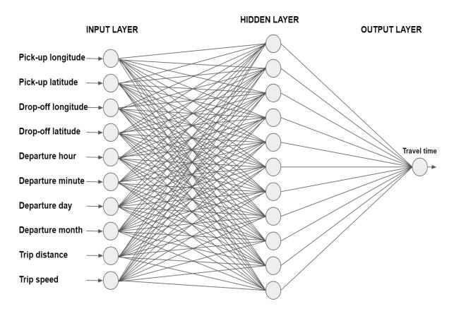
Figure 14: Artificial Neural Network (ANN) Model Architecture
