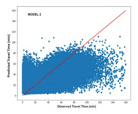
Figure 71: Convolutional Neural Network (CNN) models 2 training and validation correlation
