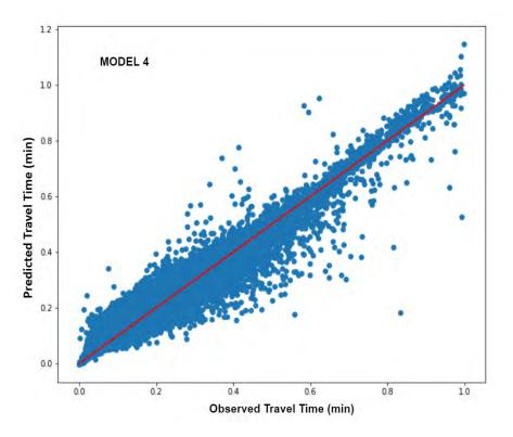
Figure 93: Long Short-Term Memory (LSTM) model 4 training and validation correlation
