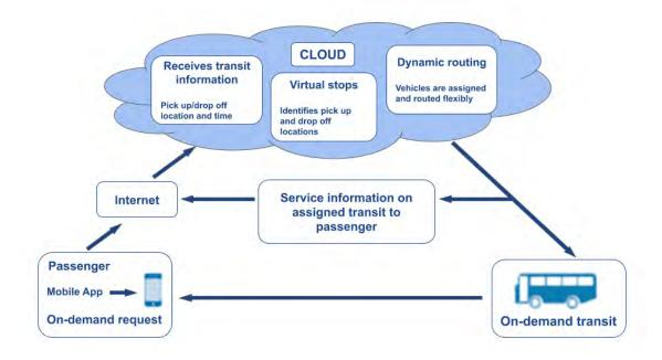
Figure 2: On-demand transit request flow, adapted from (Liyanage and Dia, 2020)
