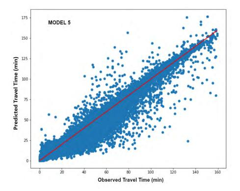
Figure 74: Convolutional Neural Network (CNN) models 5 training and validation correlation
