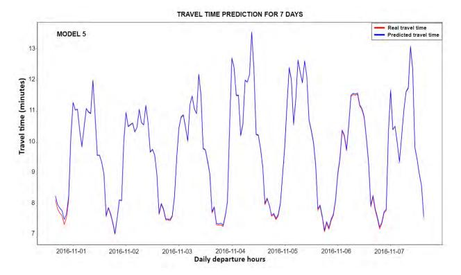
Figure 104: Long Short-Term Memory (LSTM) model 5 travel time prediction per hour
