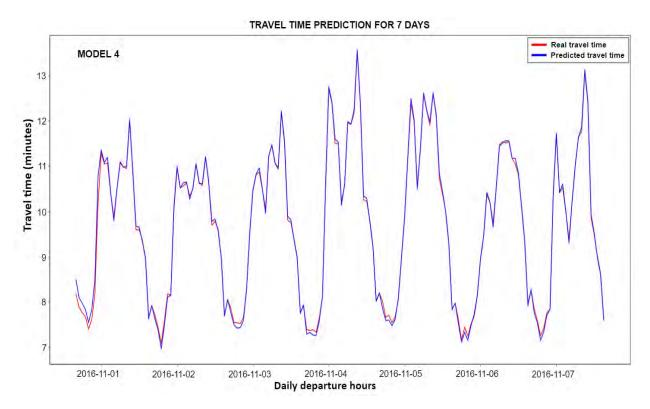
Figure 103: Long Short-Term Memory (LSTM) model 4 travel time prediction per hour
