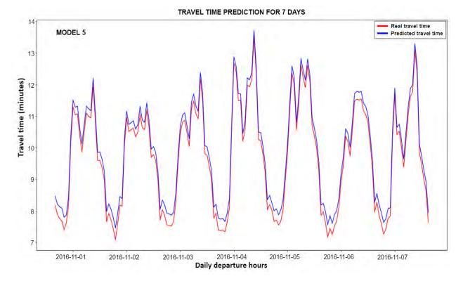
Figure 64: Artificial Neural Network (ANN) models 5 travel time prediction per hour
