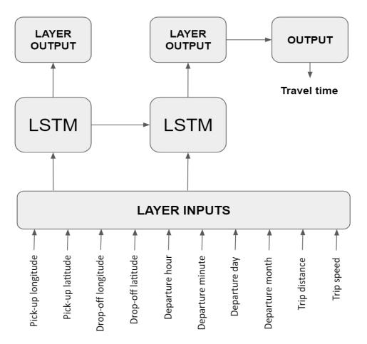
Figure 16: Long Short-Term Memory (LSTM) Model Architecture
