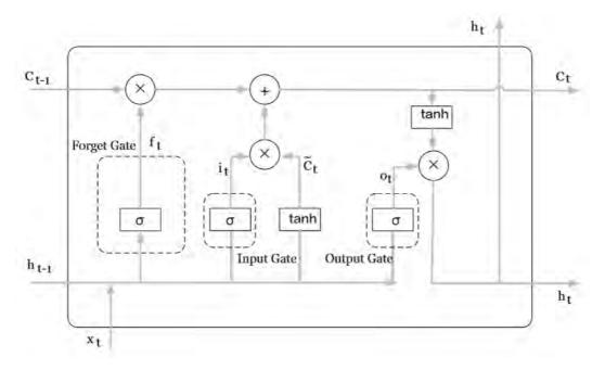
Figure 9: A Structure of LSTM Cell (Wei et al., 2018)
