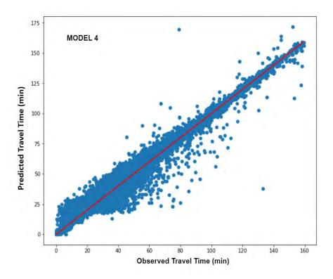
Figure 73: Convolutional Neural Network (CNN) models 4 training and validation correlation
