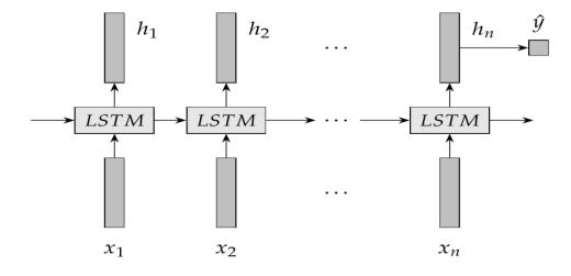
Figure 10: An architecture of LSTM Neural Network for travel time prediction (Ran et al., 2019a)
