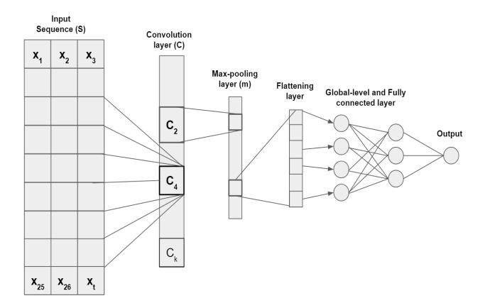
Figure 8: Convolutional Neural Network (CNN) Architecture for spatio-temporal data of travel time prediction, adapted from (Ran et al., 2019b)
