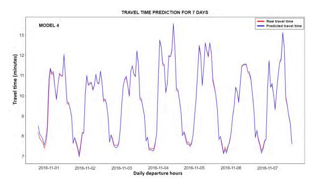
Figure 115: Long Short-Term Memory (LSTM) model 4 real travel time prediction per hour
