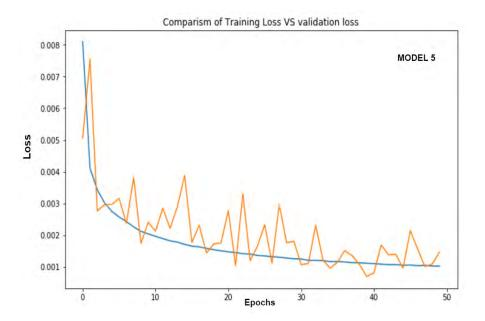
Figure 108: Long Short-Term Memory (LSTM) model 5 training and validation loss curves
