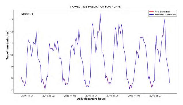
Figure 114: Convolutional Neural Network (CNN) model 4 real travel time prediction/hour
