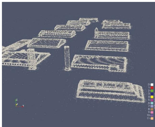
2 | CAD mesh model of Oktoberfest for CFD simulation.
