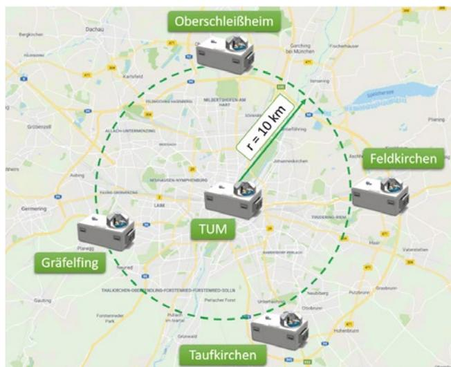
1 | Setup of the fully automated urban greenhouse gas network in Munich.
