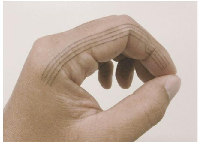
2 | Ultrathin nanomesh sensor directly applied on the finger of a human participant. These sensors are designed to measure a biological information (pressure, temperature, strain, etc).
