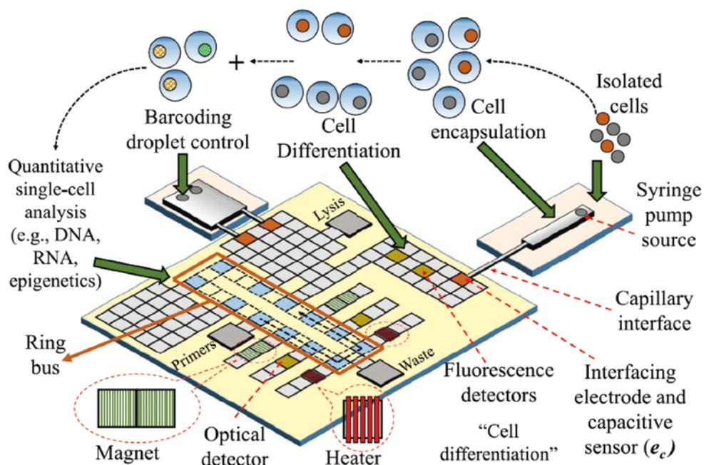
1 | Hybrid platform for single-cell analysis with a flow-based biochip for cell encapsulation and droplet generation, a digital biochip for quantitative analysis, and a reconfigurable valve-based fabric for barcoding [3].
