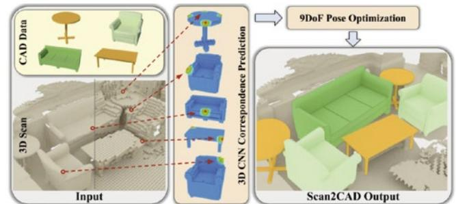
2 | Scan2CAD takes as input an RGB-D scan and a set of 3D CAD models (left). We then propose a novel 3D CNN approach to predict heatmap correspondences between the scan and the CAD models (middle). From these predictions, we formulate an energy minimization to find optimal 9 DoF object poses for CAD model alignment to the scan (right).
