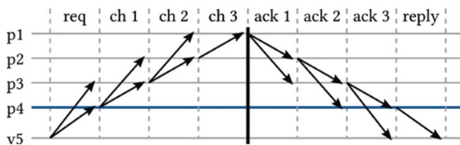
2 | Message flow of a join-request. Vehicle  $v_5$  sends the request to the platoon vehicles  $p_4$  and  $p_3$ .  $p_4$  will start a consensus round, and when  $p_1$  receives a valid chain of accepting votes, it decides for the new platoon and sends an (Ack) back to  $v_5$ .
