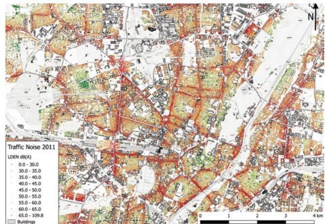
2 | Simulated noise caused by traffic in Munich
