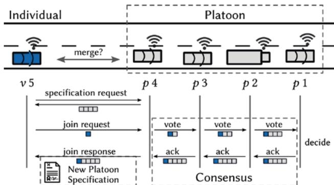
1 | Our idea of a consensus-based join maneuver. An individual vehicle requests to join an existing platoon. The join request is forwarded to each platoon vehicle, which will vote on the request. If all vehicles agree, the new vehicle is accepted and the new specification is sent to all vehicles.
