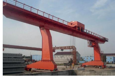
FIGURE 1: The overview of a L-type single-beam gantry crane.
