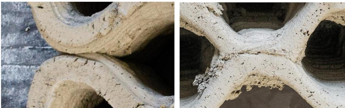
Figure 34: Weakly bonded parallel filaments with small gap in between the filaments (left) and well bonded partly overlapping filaments (right)
