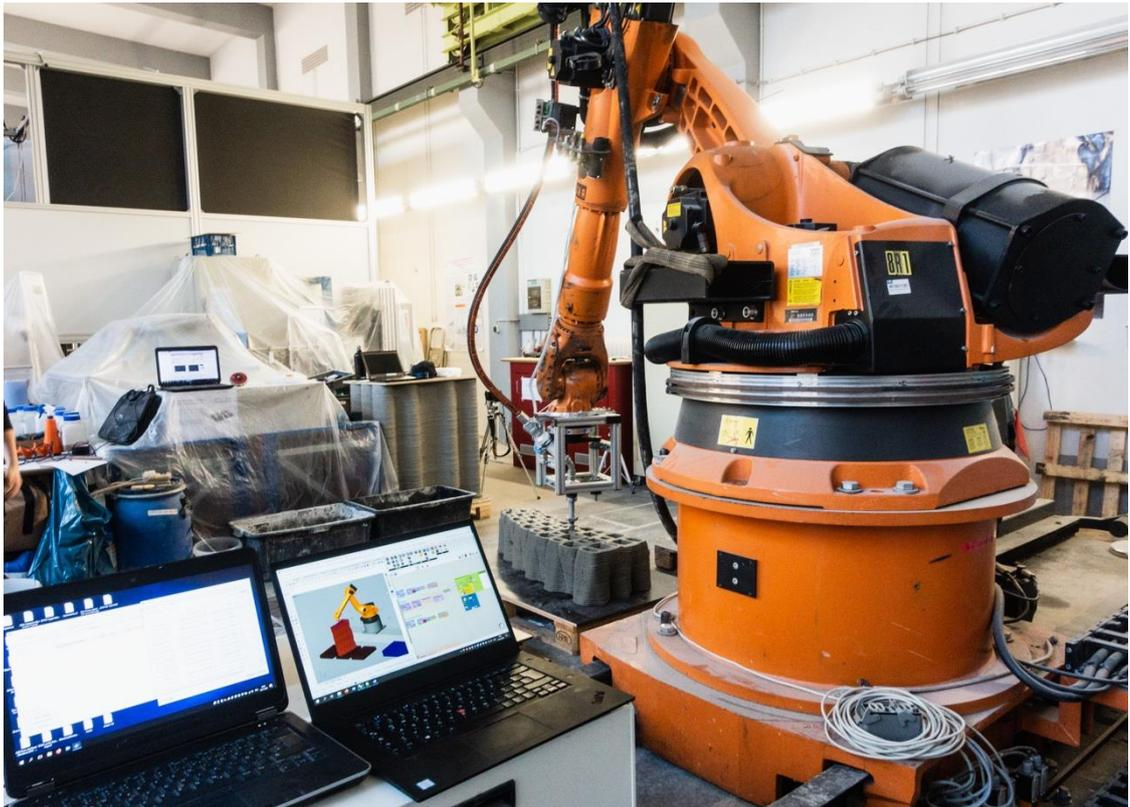
Figure 29: Robotic setup of printing process at Technical University of Munich
