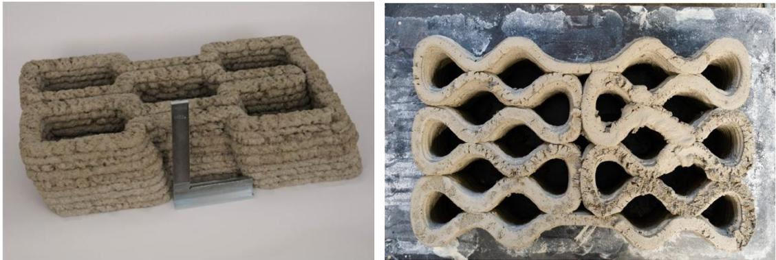
Figure 6: 3D printed wood based lightweight concrete test object showing an overhang of 26% (left) and lightweight concrete test object with internal voids (right) (Henke, Talke and Winter, 2017)
